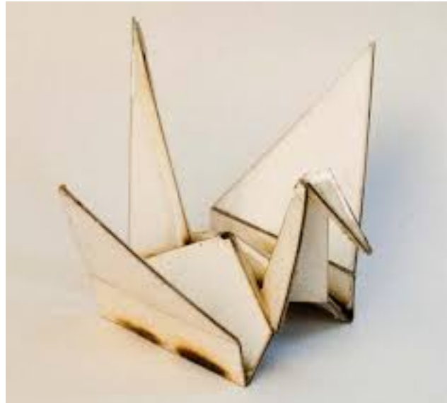
FIGURE 1.23: Self-folding crane using an electric field induced technique. The device starts as a flat composite containing several layers: structural layers, shape memory polymer layer, and a copper circuit etched onto a polyimide layer. The self-folding of the device caused by joule heating requires three minutes in order to reach the fully folded state [Felton et al., 2013b].
