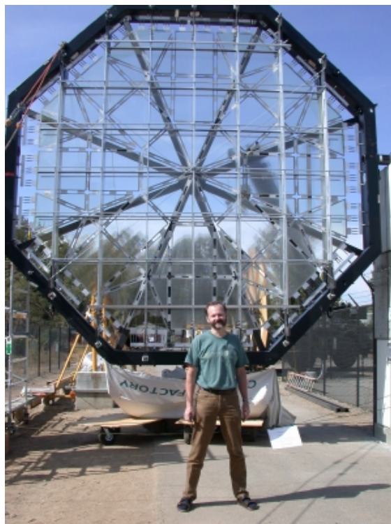
FIGURE 1.3: Prototype of the origami-based lens on its test range for the solar system's largest telescope project by the name of Eyeglass [Lang, 2015].
