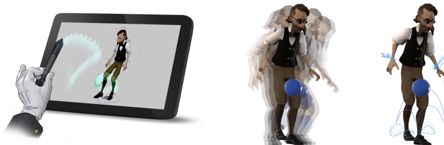
Figure 2.55: Motion cycles [CGNS17]: the user draws several loops (left), a looping motion cycle is extracted from the noisy input (middle); the user can combine different motions to create a complex animation (right).
