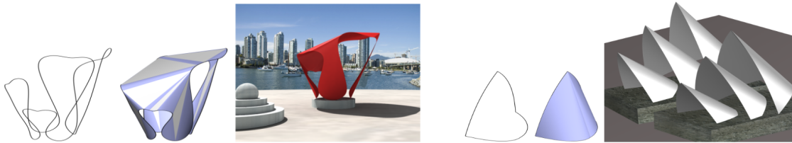
Figure 2.11: Architectural designs modelled with developable surfaces [RSW*07]: (left) gazebo; (right) Opera House.
