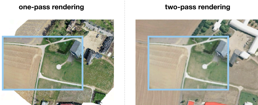
Figure 4.14: Visualization of a photograph in two different 3D scene models. A one-pass rendering is used for point clouds, while a two-pass is used for meshes.
