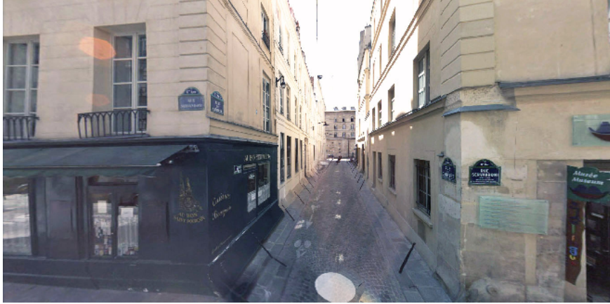
Figure 2.38: Real-time projective multi-texturing with occlusion handling using a mix of point clouds and meshes. The viewer is capable of navigating inside a scene textured only by photos (Devaux and Brédif 2016). Credits to iTowns .
