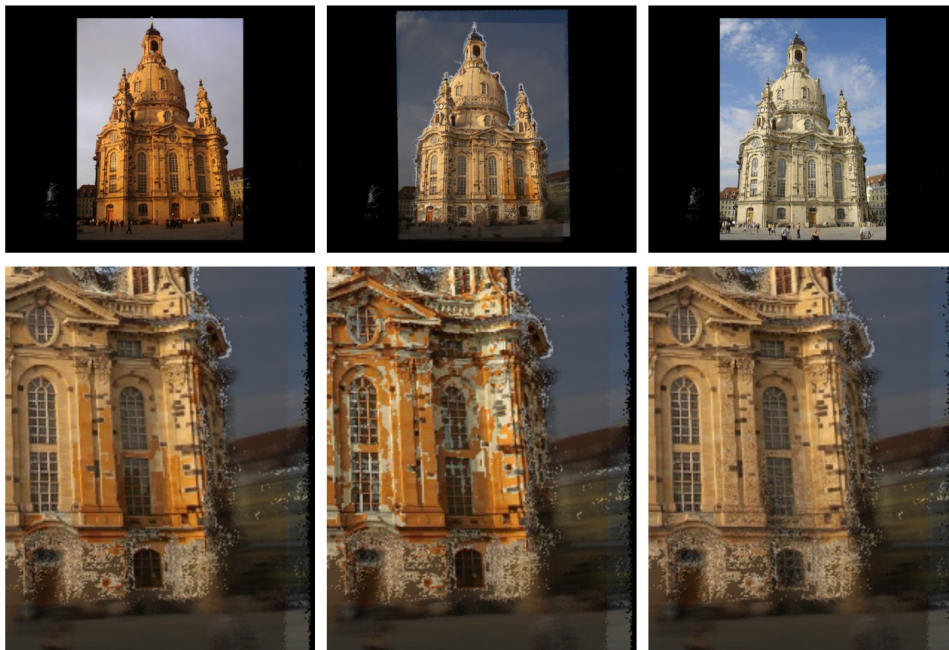
Figure 2.49: Lighting changes in the Church (Italy) dataset. Top: transition at 0%, 50%, and 100% transition time. Bottom: close-up at 50% with soft z-buffer and alpha normalization (left), without soft z-buffer (middle), and without alpha normalization (right) (Goesele et al. 2010).
