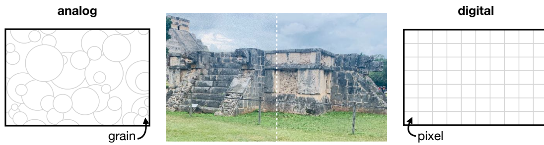
Figure 2.7: Comparison between analog and digital photography. Film (used in analog cameras) employs disperse grains of silver, and digital sensors (related to digital cameras) utilize pixels to represent an image. The differentiating photograph has been captured in Chichén Itzá (Mexico).
