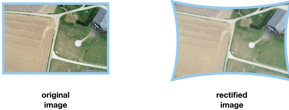
Figure 4.2: Aerial photograph with a strong distortion and its rectified version after the distortion has been removed.
