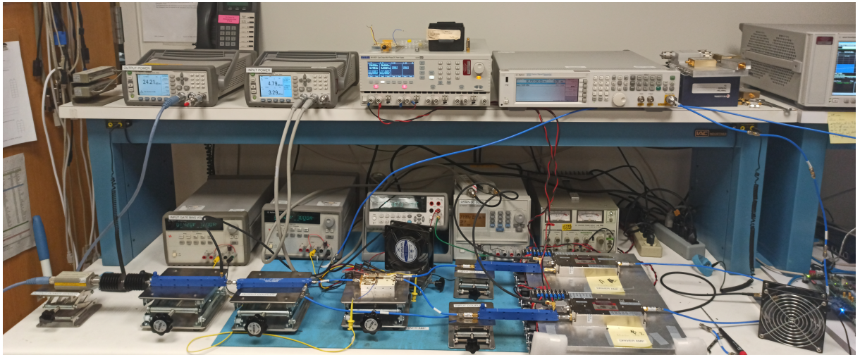
Figure 5.5: Photo of testbench of dual-input Doherty PA
