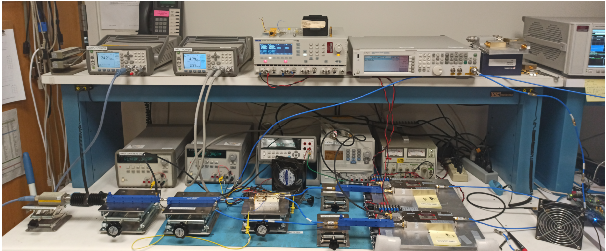
Figure 5.5: Photo of testbench of dual-input Doherty PA
