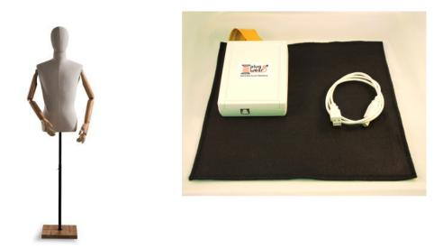
FIGURE 4.7 – The matrix sensor (right side) render position and pressure data when touched. Four matrix sensors are placed on the mannequin left arm, chest, left shoulder and back. The purpose of the mannequin-sensor is to collect social touch data from various regions of the body simultaneously.
