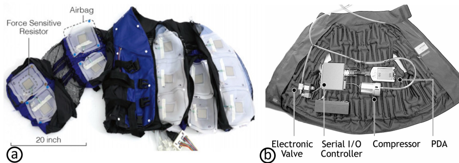
Figure 2.10: Two pneumatically-actuated jacket designs. (a) Delazio et al. created a pneumatically-actuated jacket to generate an embodied haptic experience on upper body [44]. (b) Mueller et al. created Hug Over a Distance vest to simulate touch sensation [148].
