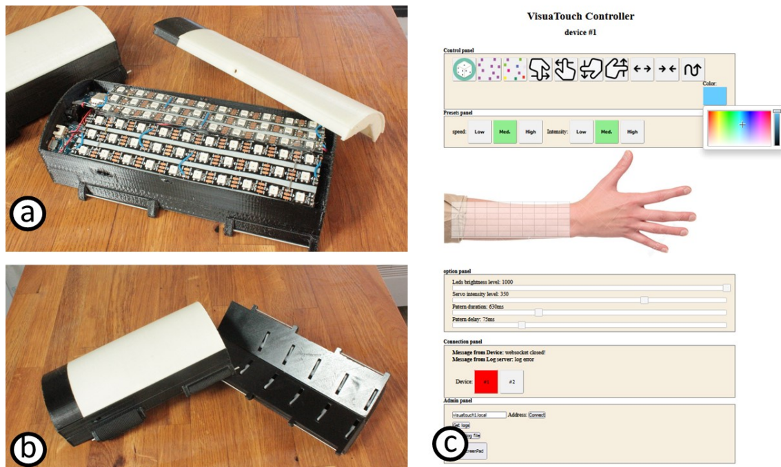
Figure 3.6: Second round iteration of VisualTouch . (a) The two layers are placed into the 3D printed case to ensure stability. (b) Alternative tactile actuation with 5 * 2 servo motors. (c) Final user interface of VisualTouch .
