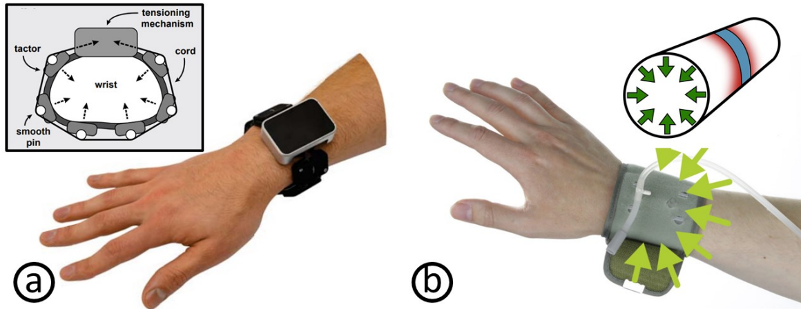
Figure 2.18: Two examples of tactile bracelets. (a) Pezent et al. designed Tasbi that supported tactile hand interactions with vibrotactile stimuli and squeeze force [169]. (b) Pohl et al. used pneumatic actuators in the Squeezeback design to generate a uniform squeeze pressure on the wrist [173].
