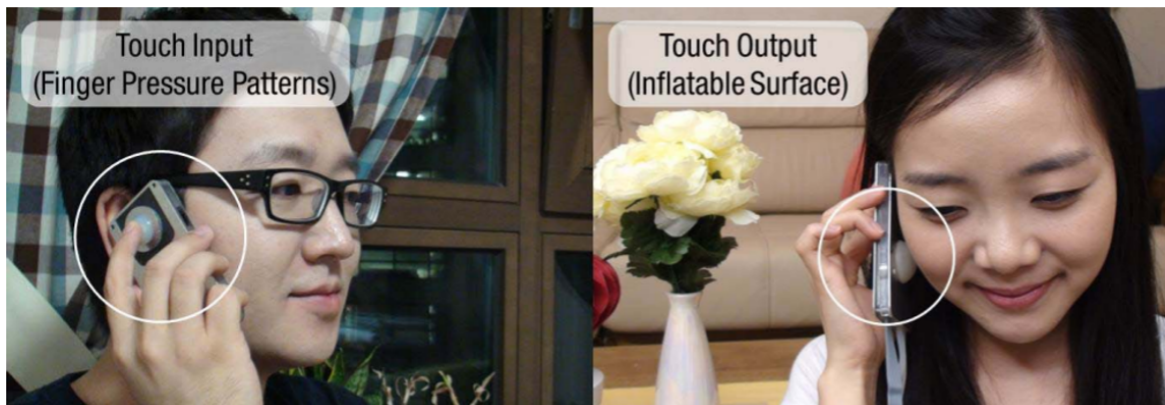
Figure 2.14: Park et al. used POKE device to enable cheek-touching interaction during the phone call [164]. During a phone call, one user (left) touch the silicon button as input, while another user (right) perceives the touch output on his/her cheek.
