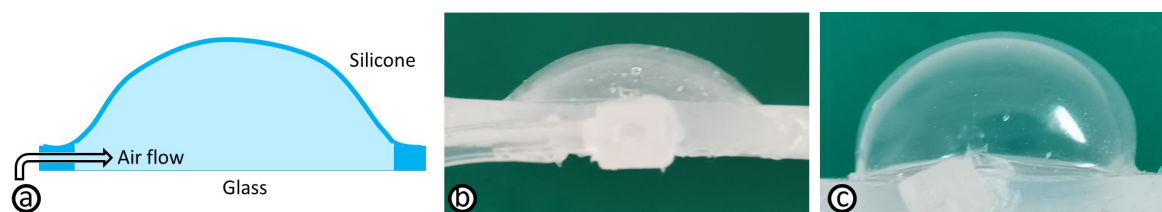
Figure 5.8: Composite structure of the airbags. (a) Two-layer structure. (b) Uni-directional inflation with 1.5mm thick silicone layer. (c) Inflation with 0.8mm thick silicone layer.
