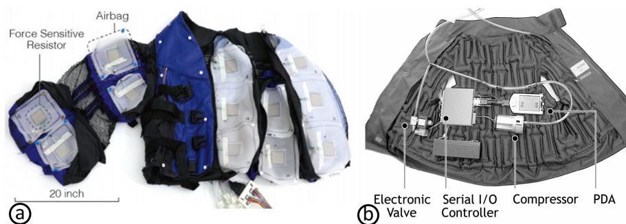
Figure 2.10: Two pneumatically-actuated jacket designs. (a) Delazio et al. created a pneumatically-actuated jacket to generate an embodied haptic experience on upper body [44]. (b) Mueller et al. created Hug Over a Distance vest to simulate touch sensation [148].
