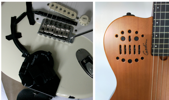
(a) Roland GK-3 installé sur la Fender Made in Japan.
