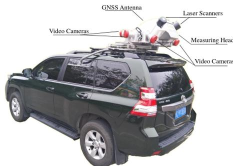
FIGURE 2.19 – Véhicule ApolloScape (HUANG et al., 2019)
