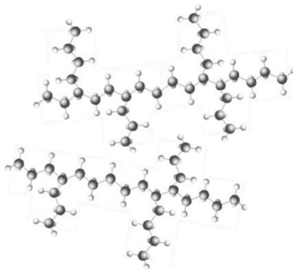
Figure 1.3: An atomic representation of short branched low-density polyethylene. Image taken from Ref. [5].
