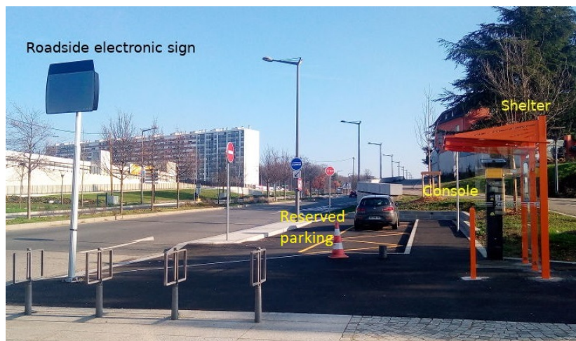
Figure 3.5 – Configuration of a physical meeting point for the 'Lane' carpooling service. The orange structure is like a bus shelter. A passenger notifies potential drivers of their carpooling request using the console, which is then displayed on the roadside electronic sign. A driver can safely embark the passenger in the reserved parking place. Reproduced with permission from Ecov.
