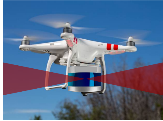
(b) A quadrotor carrying a lidar
