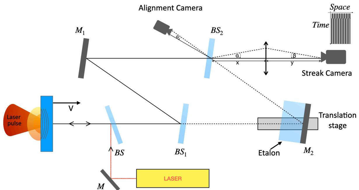
Figure 3.1: Modified Mach-Zehnder interferometer implemented on VISAR diagnostic system: the probe beam is reflected from the target rear side, the tilted  $M_2$  mirror results in the formation of fringes on the alignment camera after recombination of the two images from the two arms of the interferometer.
