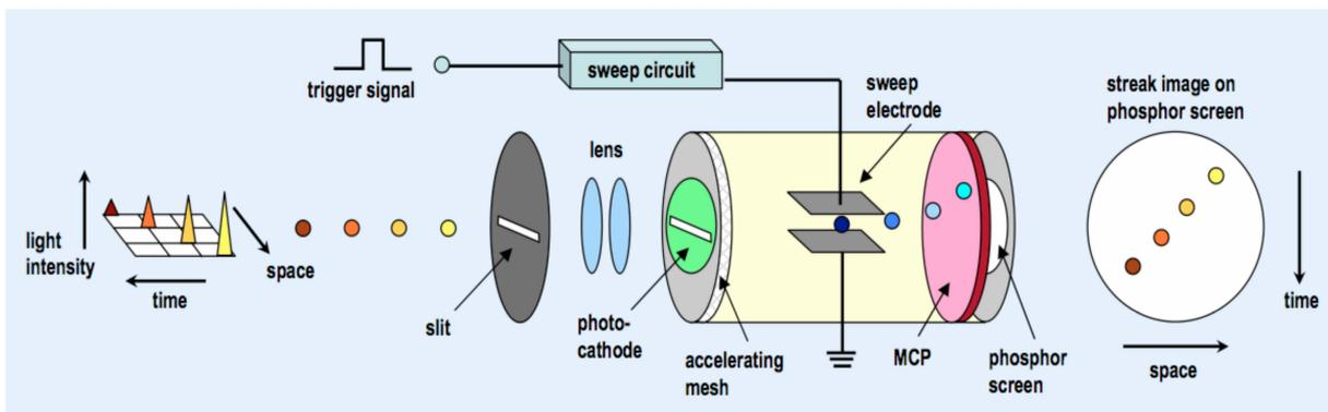
Figure 3.7: Operating principle of a streak tube. Source: [www.hamamatsu.com](http://www.hamamatsu.com).
