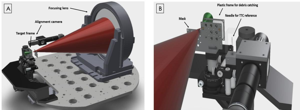
Figure 7.2: CAD design for PALS drive beam and the specially designed motorised target holder suitable for HRR experiment taking into account the real size of the beam and the chamber space. (A) Side view of the target frame and the focusing lens and (B) Front view of the target holder where we highlight the needle target for setting a reference point on the TCC, the mask in front of the target holder and the plastic frame placed to protect optics from debris.
