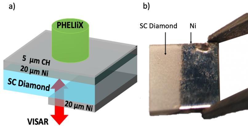
Figure 4.3: a) scheme of the target used in the experiment, b) image of Ni layer deposited on target rear side (taken before deposition of Ni layer on target front side).
