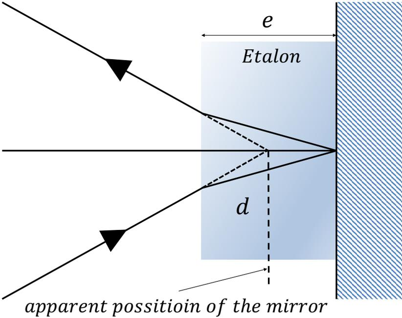
Figure 3.2: Correction of the mirror position after the insertion of the etalon on one arm of the interferometer.
