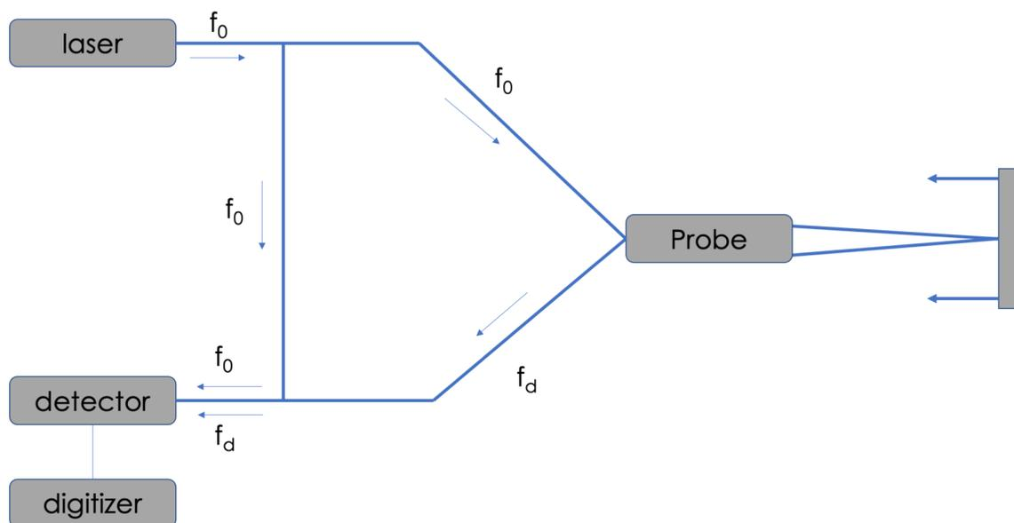
Figure 7.10: PDV velocimeter working principle
