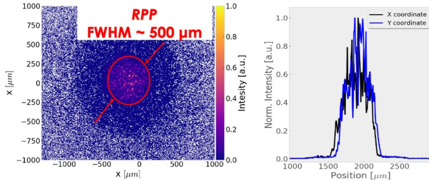
Figure 4.2: Experimental optimisation of the intensity profile of the PHELIX GSI laser facility using Random Phase Plate to produce  $\sim 500 \mu\text{m}$  Gaussian spot. [left] Effect of the RPP normalised and background removal, [right] line out along  $x$  and  $y$  axis after fitting a gaussian function we get a  $FWHM \sim 500 \mu\text{m}$ .
