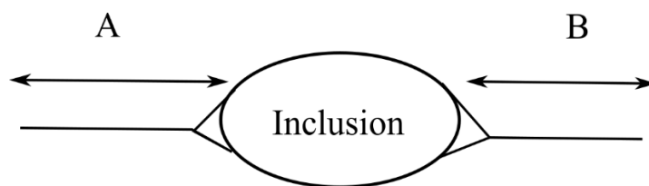
Figure 873: Measurement of the size of cracks induced around an inclusion
