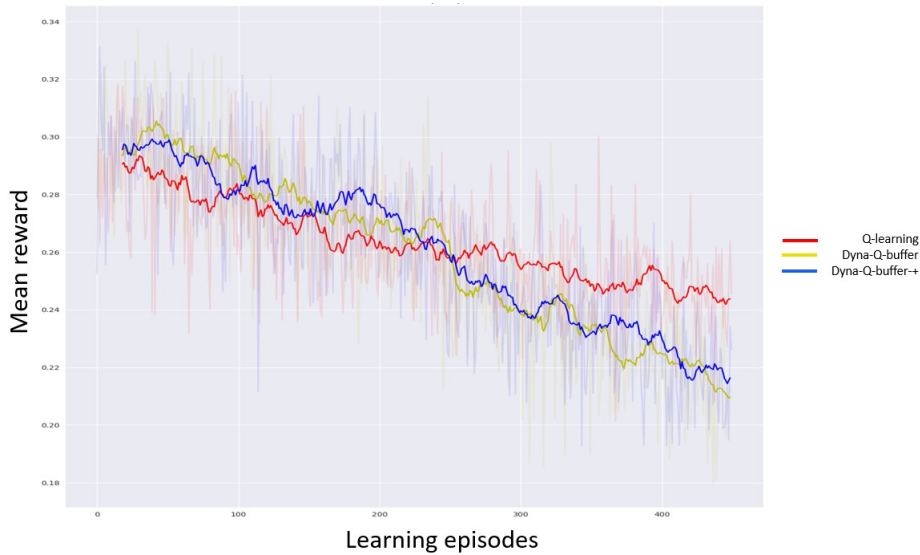
FIGURE 5.3 – Average reward over learning episodes in tandem queue environment with larger scale
