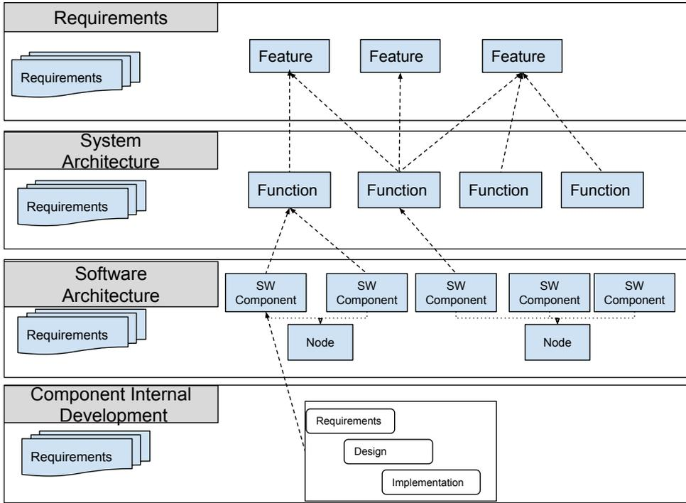
Figure 2.1: Component-Based Software Development Process and Used Artifacts [10]
