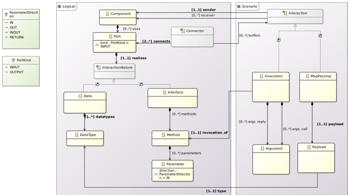
Figure 4.3: Component-port-connector meta-model
