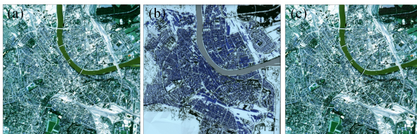
Figure 4.8 (a) PlanetScope image in the Basel area. (b) DART image simulated with constant SS per urban component. (c) DART image after the calibration procedure. All images are RGB colour composites.
