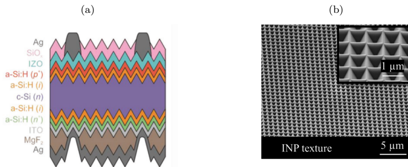
Figure 1.10: (a) Schematic of the infrared-enhanced SHJ cell [66]. (b) Periodic INP gratings of 800 nm pitch were fabricated by NIL [70].
