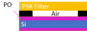
Figure 7.8: Scheme of perovskite filter mechanically stacked on the masked Silicon cell associated.
