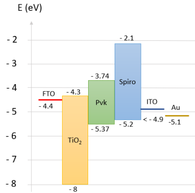
Figure 3.3: Energy band diagram of reference STPC with an ITO electrode on the back side [219–221].
