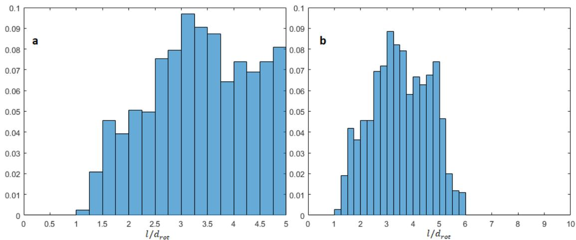
Figure 5.8. Distribution of the interparticle spacing in the case of *PNT57* particles for  $Re = 116$  and  $X/H = 1000$ , for two different values of the critical interparticle spacing ((a)  $5d_{rot}$  and (b)  $10d_{rot}$ ). The y-axis represents the number of spacings over the total number of spacings. The x-axis corresponds to the normalized interparticle spacing ( $l/d_{rot}$ ).
