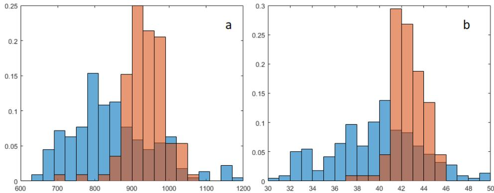
Figure 4.5. (a) Surface area  $A$  and (b) rotational diameter  $d_{rot}$  distribution of visually identified tumbling (red) and non-tumbling particles (blue). The x-axis is in pixels and the y-axis corresponds to the number of particles over the total number of particles.
