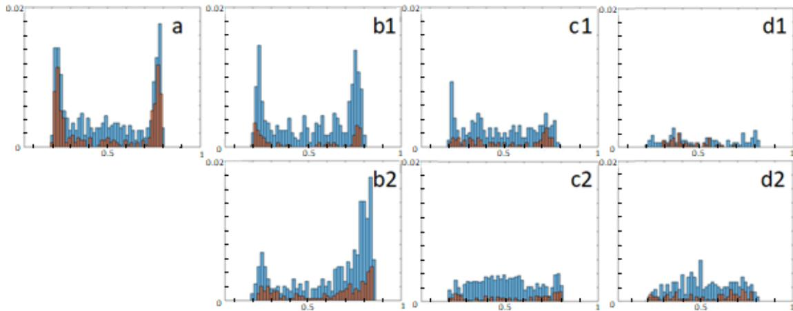
Figure 4.7. Histograms representing the distributions of bright PNT57 particles (blue) and in-plane bright tumbling particles (red) at different channel depths: (a) midplane (b1) and (b2)  $Z/H = 0.625$  and  $0.375$ ; (c1) and (c2)  $Z/H = 0.75$  and  $0.25$ ; (d1) and (d2)  $Z/H = 0.875$  and  $0.125$ . The x-axis represents  $Y/H$  and the y-axis varies between 0 and 0.02.
