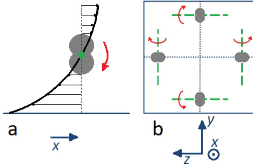
Figure 4.4. The tumbling behavior of focused elongated particles ( $\lambda > 1$ ) in a square microchannel, observed from (a) the longitudinal and (b) the lateral cross-sections. The green dot in (a) and the dashed green lines in (b) represent the rotational axes. The red arrows correspond to the sense of rotation.
