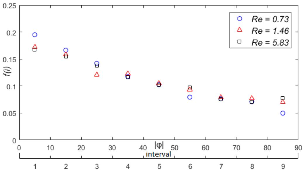
Figure 4.10. The orientation distribution for three different values of Reynolds number, at  $X/H = 7125$ . On the x-axis, the nine intervals are present. On the y-axis, the fraction of particles  $f(i)$  is found.
