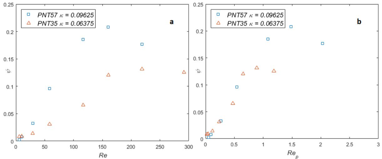
Figure 5.4. Evolution of the fraction of particles in trains  $\psi$  in function of (a) the channel Reynolds number and (b) the particle Reynolds number, for *PNT35* ( $\kappa = 0.06375$ , red triangles) and *PNT57* ( $\kappa = 0.09625$ , blue square) particles. Both suspensions have the same number of particles ( $\Phi_{eq} = 0.1\%$ ) and the tests are done at  $X/H = 1000$ .
