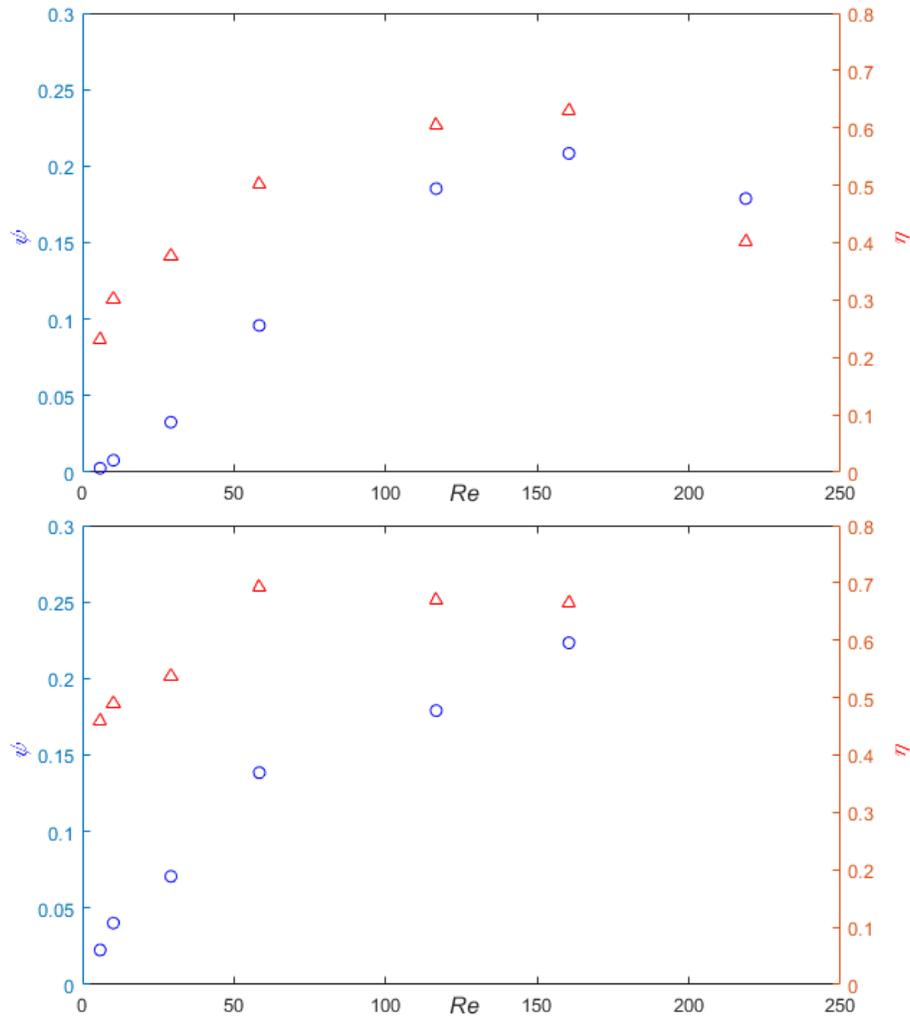
Figure 5.2. Evolution of the fraction of particles in trains  $\psi$  (blue circles, left y-axis) and the focusing degree  $\eta$  (red triangles, right y-axis) in function of Reynolds number, for PNT57 (up) and SNW (down) particles.
