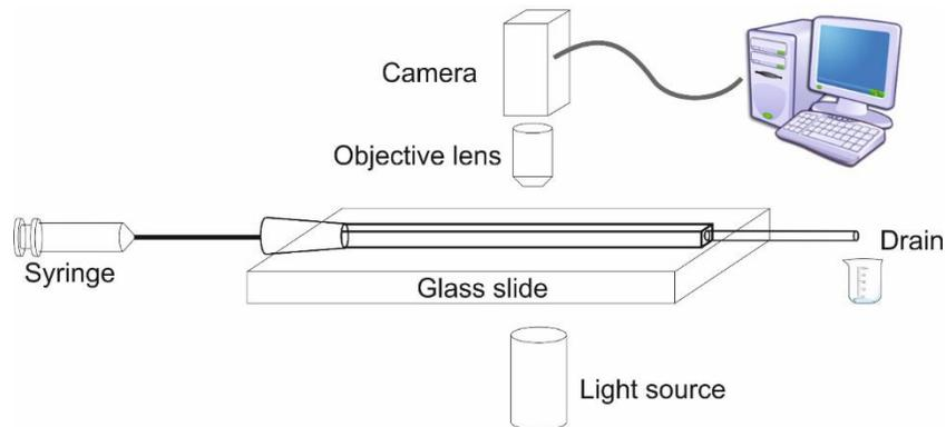
Figure 2.2. Experimental setup of the *in-situ* visualization method [67].
