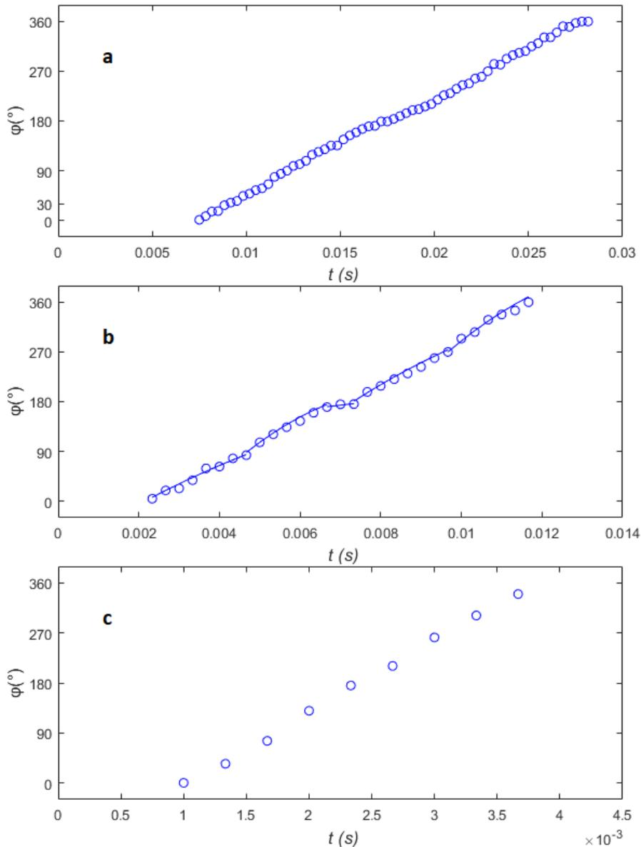
Figure 4.8. Evolution of the orientation of a SNW particle in function of time, at (a)  $Re = 0.73$  (up), (b)  $1.46$  (center) and (c)  $5.84$  (down). The tests are done on the same suspension, at  $X/H = 1000$ .
