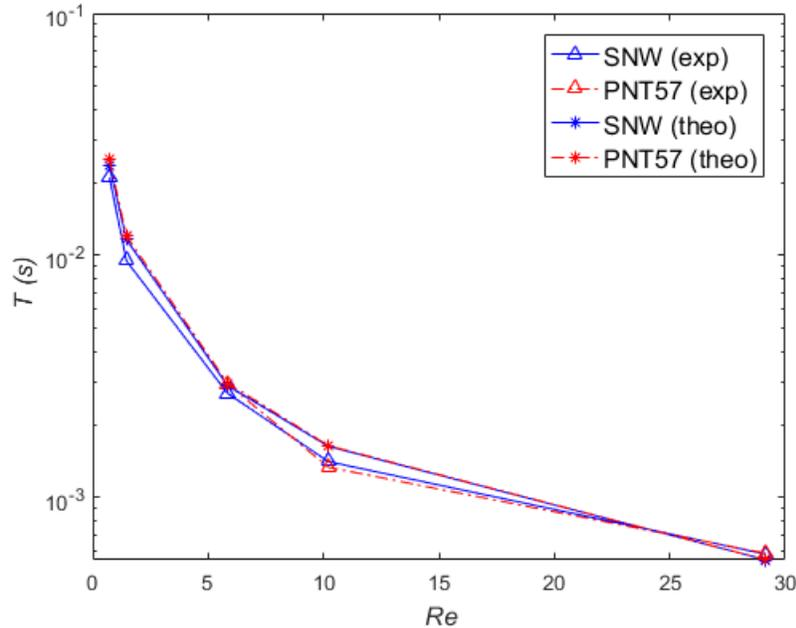
Figure 4.13. Experimental and theoretical periods of rotation as a function of Reynolds number, for two types of particles (SNW and PNT57). The experimental tests are done at  $X/H = 1000$ . The maximum error in the measured period of rotation is equal to  $3.3 \times 10^{-4} s$ .
