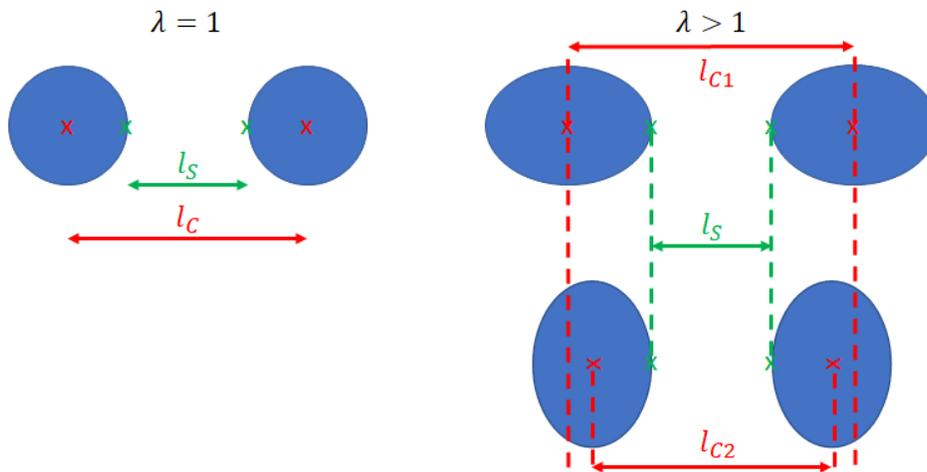
Figure 5.9. The distances  $l_S$  and  $l_C$  between two consecutive particles in a train, for  $\lambda = 1$  and  $\lambda > 1$ .
