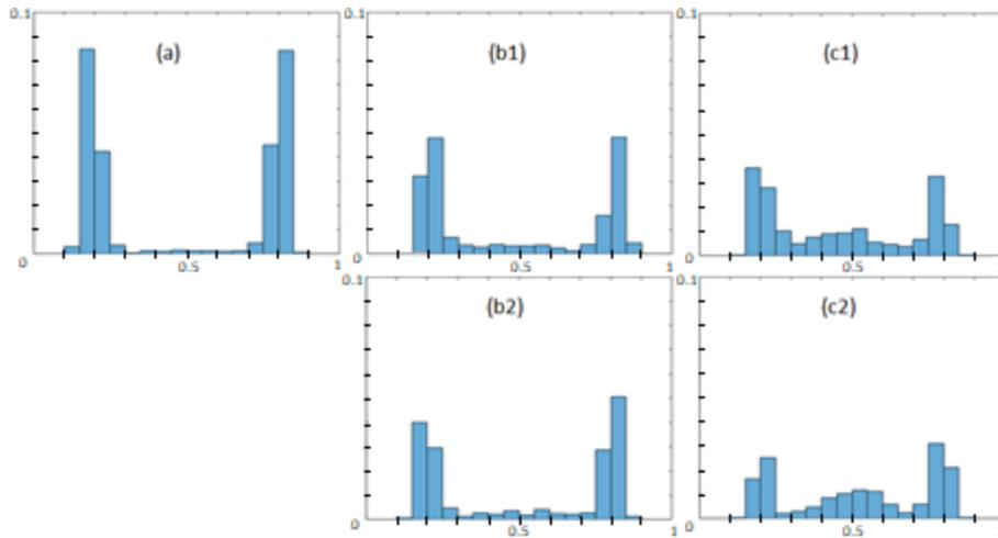
Figure 5.3. Histograms representing the distributions of bright PNT57 particles in trains, at  $Re = 5.83$  and different channel depths: (a) midplane (b1) and (b2)  $Z/H = 0.75$  and  $0.25$ ; (c1) and (c2)  $Z/H = 0.875$  and  $0.125$ . The x-axis represents  $Y/H$  and varies between 0 and 1. The y-axis corresponds to the fraction of bright particles in trains and varies between 0 and 0.1.
