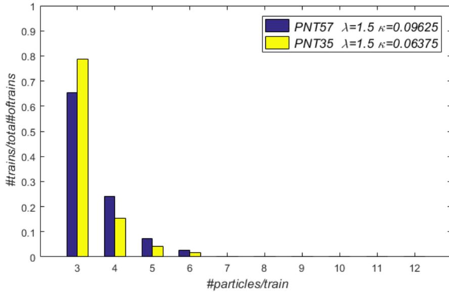
Figure 5.5. Fraction of trains as a function of the number of particles per train, for PNT57 ( $\kappa = 0.09625$ ) and PNT35 ( $\kappa = 0.06375$ ) particles, at  $Re = 58$ . Both suspensions have the same equivalent concentration ( $\Phi_{eq} = 0.1\%$ ).
