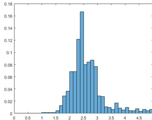
Figure 5.7. Example of the distribution of the normalized interparticle spacing in the case of *SNW* particles, flowing at  $Re = 160$  and  $X/H = 750$ . The y-axis represents the number of spacings over the total number of spacings. The x-axis corresponds to the normalized interparticle spacing ( $l/d_{rot}$ ).
