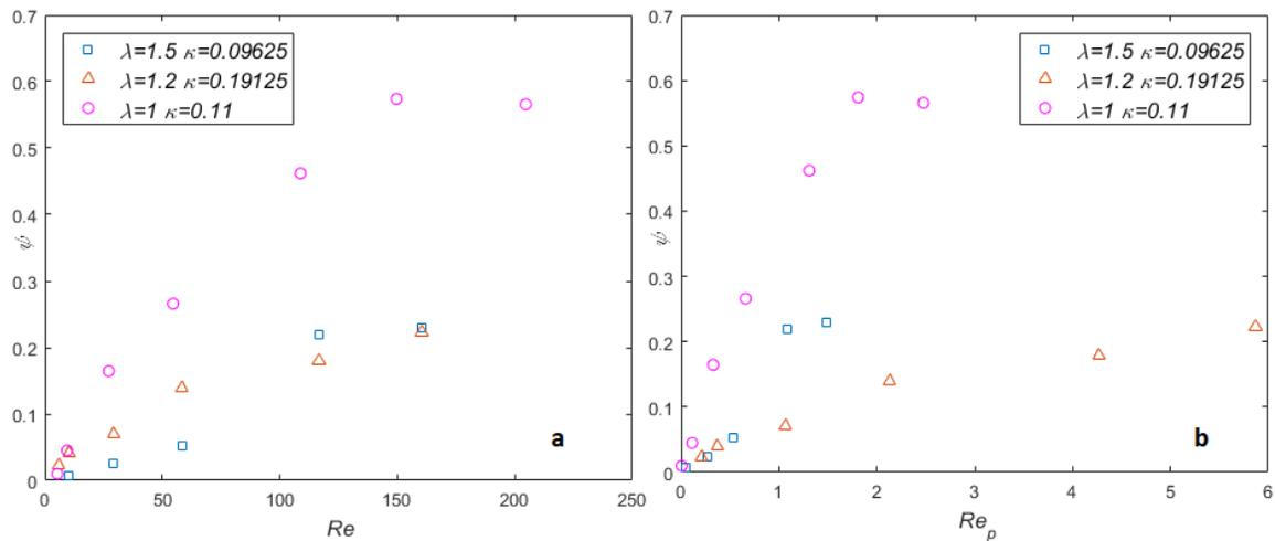
Figure 5.6. Evolution of the fraction of particles in trains  $\psi$  in function of (a) the channel Reynolds number and (b) the particle Reynolds number, for PNT57 ( $\kappa = 0.09625, \lambda = 1.5$ , blue square), SNW ( $\kappa = 0.19125, \lambda = 1.2$ , red triangle)
