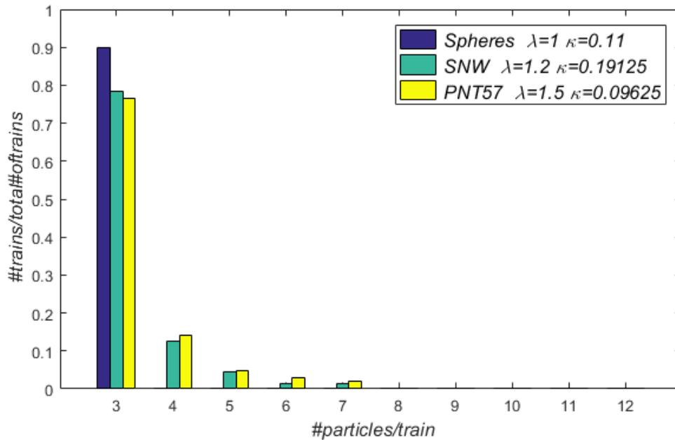
Figure 5.10. Fraction of trains as a function of the number of particles per train, for SNW ( $\kappa = 0.19125$ ,  $\lambda = 1.2$ ), PNT57 ( $\kappa = 0.09625$ ,  $\lambda = 1.5$ ), and spherical [67,93,159] particles. All the suspensions have the same equivalent concentration ( $\Phi_{eq} = 0.05\%$ ), and flowing at  $Re = 58$ .
