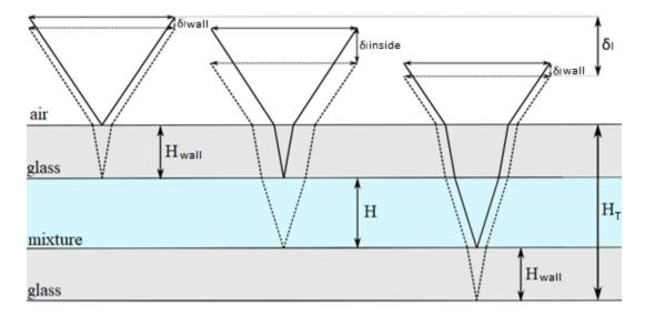
Figure 2.8. Schematic representing the link between the channel displacement and that of the focal plane.
