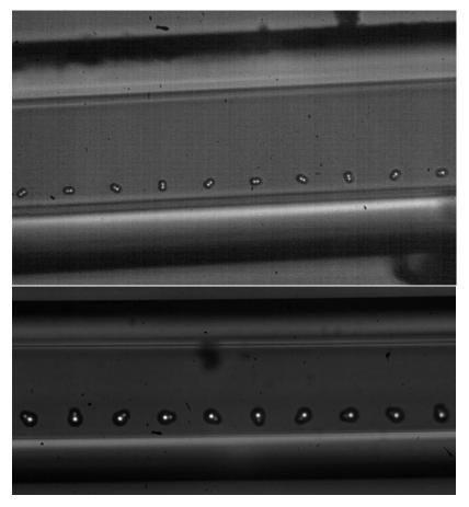
Figure 4.1. The tumbling mode of two focused bright tumbling PNT57 (up) and SNW (down) particles, at Re = 5.84 and Z/H = 0.5. These figures are obtained by superposing 10 consecutive images with the background. The suspension is flowing from left to right.
