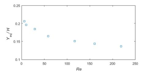
Figure 3.8. Normalized equilibrium position in function of the channel Reynolds number. The suspension contains PNT57 particles at an equivalent volume fraction of 0.1% and the tests are done at X/H=1000.
