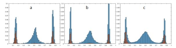
Figure 3.9. Midplane PDFs of a PNT57 suspension at different particle volume fractions: (a) 0.0175%, (b) 0.035% and (c) 0.07%. The suspension is flowing at Re = 160 and the test is done at X/H = 500. The horizontal axis varies between 0 and 1, while the vertical axis varies between 0 and 0.1 (10%).
