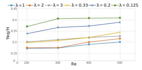
Figure 1.18. The results of Huang et al. [148] represented as the evolution of the normalized equilibrium position of an ellipsoidal particle (prolate and oblate) as a function of the Reynolds number. H is the channel's height.
