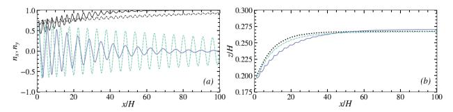
Figure 1.15. (a) x-components (colored curves) and y-components (black curves) of the orientation vector of an oblate and (b) trajectories for spheroids with  $\kappa = 0.15$  and  $\lambda = 0.5$  (solid), 0.8 (dashed), and 1 (dotted). Reprinted from [109].
