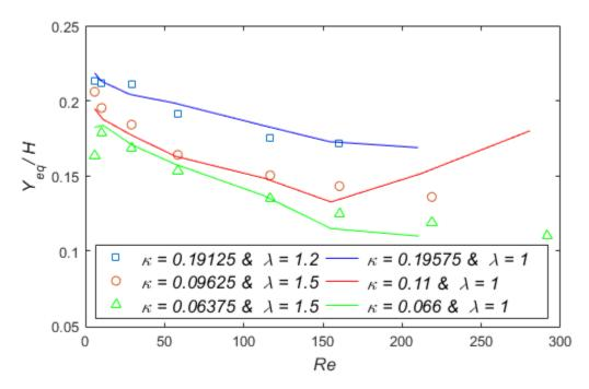
Figure 3.13. Normalized equilibrium position in function of the channel Reynolds number for spherical (lines) [93] and non-spherical particles (symbols). All the suspensions have the same number of particles ( $\Phi_{eq}=0.1\%$ ) and the tests are done at X/H=1000 in an  $80\mu m$  square microchannel.
