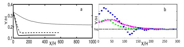
Figure 3.5. Normalized lateral position in function of the normalized distance from the inlet for (a) spherical [53] and (b) oblate particles [108]. It can be observed that once the particle is focused at a fixed Y/H, it maintains this equilibrium position regardless of the value of X/H. Figures a and b are reprinted from [53] and [108] respectively.
