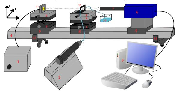
Figure 2.5. Schematic illustration of the experimental apparatus: (1) the light source, (2) the syringe pump, (3) the computer with the corresponding software, (4) the rail, (5) the rail carriages, (6) the camera, (7) the optic tube, (8) the linear stages and their micrometer heads, (9) the lab jacks, (10) the drain, (11) the optical mount, (12) the 90° angle bracket (on which the channel is fixed) and (13) the bench legs.
