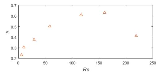
Figure 3.7. Focusing degree in function of the channel Reynolds number for PNT57 particles ( $\lambda=1.5$  and  $\kappa=0.09625$ ). The equivalent particle volume fraction is 0.1% and the tests are done at X/H=1000 in an 80 $\mu$ m square microchannel.
