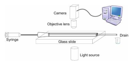
Figure 2.2. Experimental setup of the in-situ visualization method [67].
