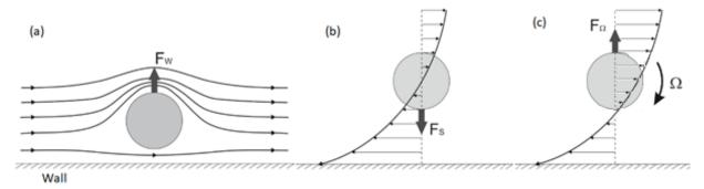
Figure 1.5. Illustration of (a) the wall-induced lift force  $F_W$ , (b) the shear-induced lift force  $F_S$ , and (c) the rotation-induced lift force  $F_\Omega$ . Figures (a) and (b) are reprinted from [67].
