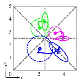
Figure 1.20. Lateral trajectories of oblate rigid particles of different sizes in a square duct at Re=100. The particles have the same aspect ratio (ratio between the particle axes,  $\lambda=1/3$ ) and different volumes. The confinement ratios  $\kappa$
