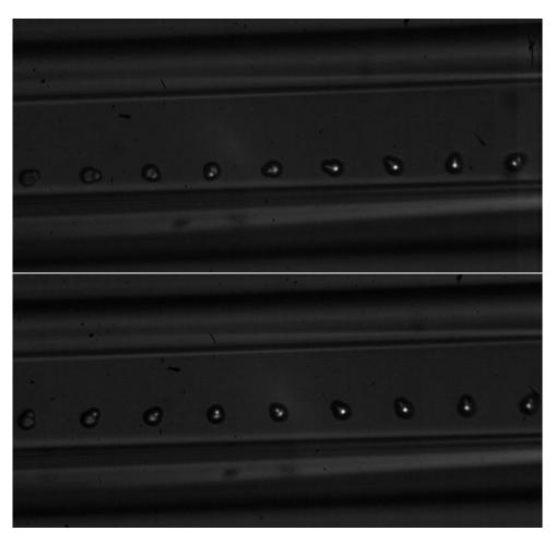
Figure 4.2. The trajectories of two SNW particles. The upper particle is focused on the ring and is in its second phase of migration. The lower particle is still in the first phase, reaching the equilibrium ring. The test is done at Re = 5.84 and Z/H = 0.625.
