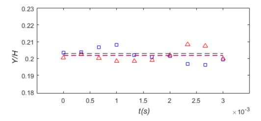
Figure 3.15. Trajectories (Y/H) of two SNW particles (red triangles and blue squares) in function of time at X/H = 1000. The suspension ( $\Phi_{eq} = 0.05\%$ ) is flowing at Re = 5.84. The normalized equilibrium position is equal to 0.203 (dashed black line). The mean values about which the particles oscillate are represented by the dashed red and blue lines, that are approximately superposed.
