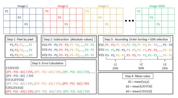
Figure 2.12. Schematic resuming the error calculation test, done for the pixels  $P_1$ ,  $P_2$  and  $P_3$ , over the 2000 images.
