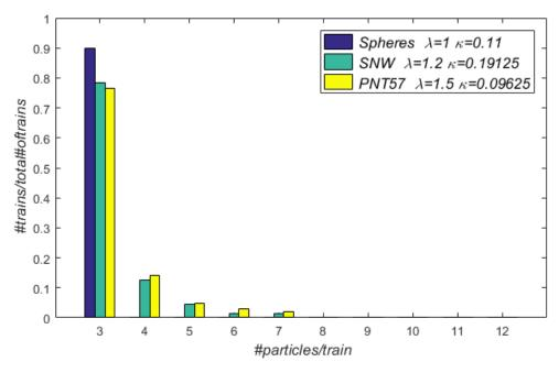
Figure 5.10. Fraction of trains as a function of the number of particles per train, for SNW ( $\kappa=0.19125,\ \lambda=1.2$ ), PNT57 ( $\kappa=0.09625,\ \lambda=1.5$ ), and spherical [67,93,159] particles. All the suspensions have the same equivalent concentration ( $\Phi_{eq}=0.05\%$ ), and flowing at Re=58.
