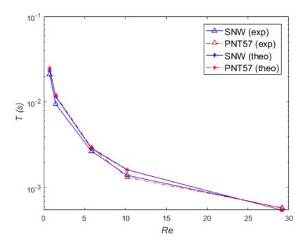
Figure 4.13. Experimental and theoretical periods of rotation as a function of Reynolds number, for two types of particles (SNW and PNT57). The experimental tests are done at X/H = 1000. The maximum error in the measured period of rotation is equal to  $3.3 \times 10^{-4}$  s.
