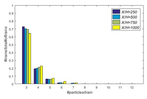
Figure 5.15. Fraction of trains as a function of the number of PNT57 particles per train, for different distances from the channel inlet, at Re = 160.
