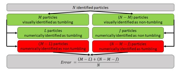
Figure 4.6. Schematic summarizing the error calculation.
