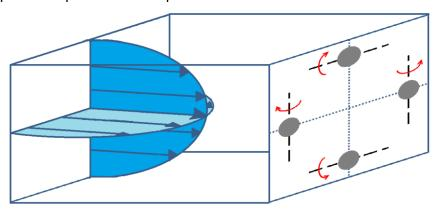
Figure 1.7. A schematic representing a square microchannel in which particles are focused on their equilibrium positions and are rotating around their rotational axis (dashed black lines).
