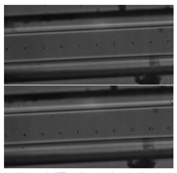
Figure 4.3. The trajectories of two PNT57 particles. The upper particle is focused on the equilibrium position and tumbling perpendicularly to the plane of the camera. The lower particle is located at the edge of the ring and having a kayaking rotational mode. The test is done at Re = 5.84 and Z/H = 0.75.
