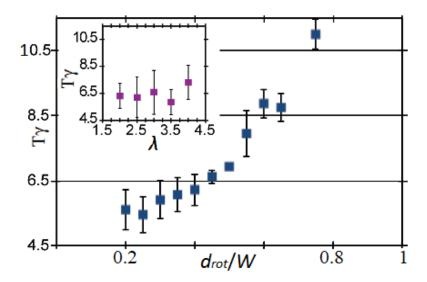
Figure 1.21. Normalized period of rotation of doublets with various size and asymmetry as a function of the aspect ratio  $\lambda$  (purple) and the confinement ratio  $d_{rot}/W$  (blue). Reprinted from [110].
