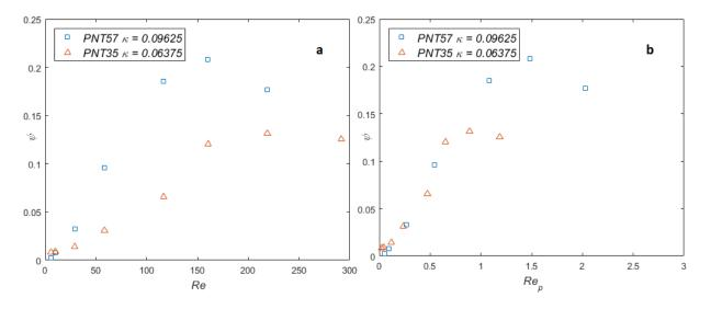
Figure 5.4. Evolution of the fraction of particles in trains  $\psi$  in function of (a) the channel Reynolds number and (b) the particle Reynolds number, for PNT35 ( $\kappa=0.06375$ , red triangles) and PNT57 ( $\kappa=0.09625$ , blue square) particles. Both suspensions have the same number of particles ( $\Phi_{eq}=0.1\%$ ) and the tests are done at X/H=1000.
