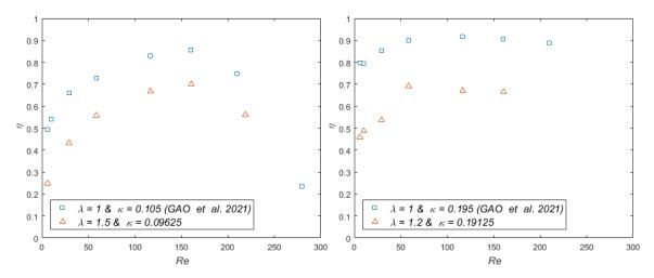
Figure 3.14. Focusing degree in function of Reynolds number for spherical (squares) [93] and non-spherical (triangles) particles. The left and right plots correspond to particles with  $\kappa \approx 0.1$  and 0.19 respectively. All the suspensions have the same number of particles ( $\Phi_{eq} = 0.05\%$ ) and the tests are done at X/H = 1000 in an 80µm square microchannel.
