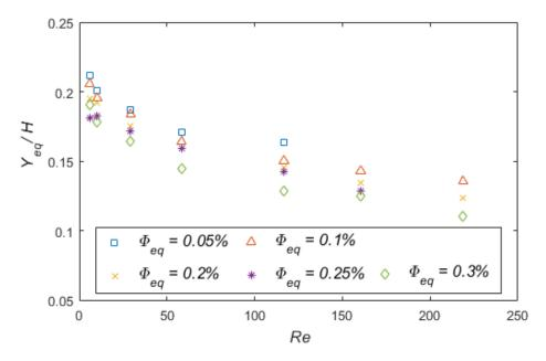
Figure 3.11. Normalized equilibrium position in function of the channel Reynolds number for different concentrations. The suspension contains PNT57 particles and the tests are done at X/H = 1000.
