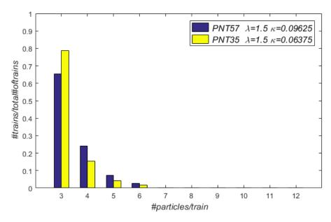
Figure 5.5. Fraction of trains as a function of the number of particles per train, for PNT57 ( $\kappa = 0.09625$ ) and PNT35 ( $\kappa = 0.06375$ ) particles, at Re = 58. Both suspensions have the same equivalent concentration ( $\Phi_{ea} = 0.1\%$ ).
