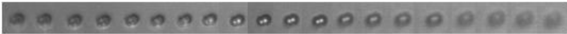
Figure 2.11. Scan of a static PNT57 ( 5.1\mu\text{m}\times 7.7\mu\text{m} ) particle in the channel. The difference between two consecutive images is equal to a lens displacement of 2\mu\text{m} . The particle appears to be non-blurry for a lens displacement corresponding to a depth of field approximately equal to 10\mu\text{m} .
