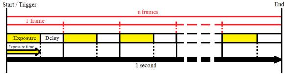
Figure 2.6. Schematic illustrating the process of image capturing during one second (FR = n fps).
