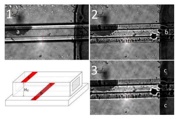
Figure 2.9. Schematic showing the three marks on the channel. The zones (a), (b) and (c) are in the plane of focus in the images (1), (2) and (3) respectively.
