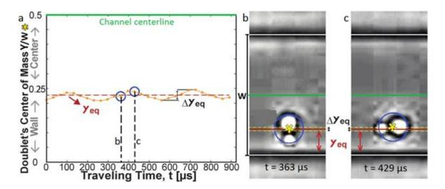
Figure 1.16. The oscillations of the center of mass of a doublet around its equilibrium position  $Y_{eq}$ . This latter is determined by averaging the values of the positions of the particle's center. Blue circles in (a) indicate the data points retrieved from the high-s speed microscopic images ((b) and (c)) taken at the corresponding times. Reprinted from [110].
