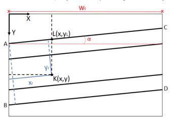
Figure 2.20. Schematic of the particle localization in the channel.
