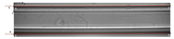
Figure 2.19. The identification of the external walls (AC and BD) as well as the inclination of the channel  $\alpha$ , using the calculated background. The orange line is horizontal, while the red line is inclined by  $\alpha$ .
