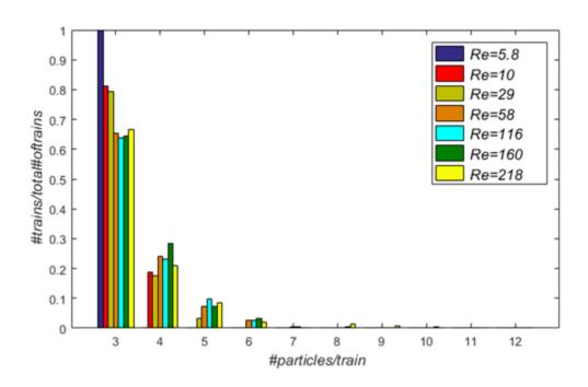
Figure 5.12. Fraction of trains as a function of the number of PNT57 particles per train, for seven values of Reynolds number.
