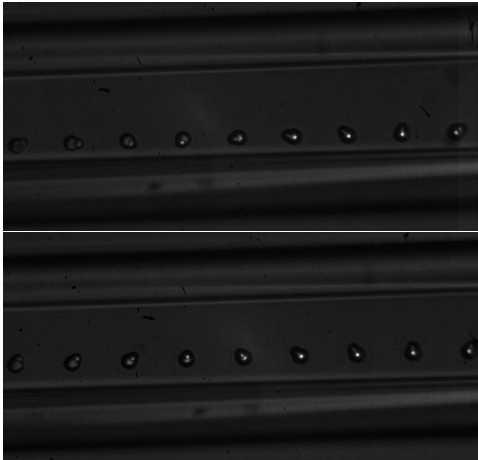
Figure 4.2. The trajectories of two SNW particles. The upper particle is focused on the ring and is in its second phase of migration. The lower particle is still in the first phase, reaching the equilibrium ring. The test is done at Re = 5.84 and Z/H = 0.625 .
