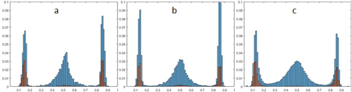
Figure 3.9. Midplane PDFs of a *PNT57* suspension at different particle volume fractions: (a) 0.0175%, (b) 0.035% and (c) 0.07%. The suspension is flowing at  $Re = 160$  and the test is done at  $X/H = 500$ . The horizontal axis varies between 0 and 1, while the vertical axis varies between 0 and 0.1 (10%).
