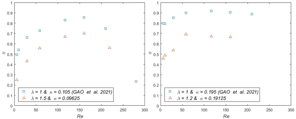
Figure 3.14. Focusing degree in function of Reynolds number for spherical (squares) [93] and non-spherical (triangles) particles. The left and right plots correspond to particles with  $\kappa \approx 0.1$  and  $0.19$  respectively. All the suspensions have the same number of particles ( $\Phi_{eq} = 0.05\%$ ) and the tests are done at  $X/H = 1000$  in an  $80\mu\text{m}$  square microchannel.
