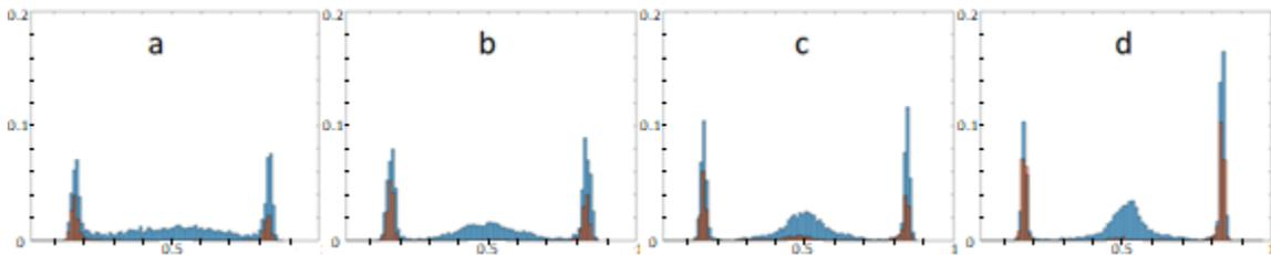
Figure 3.2. Midplane *PDFs* of a *PNT57* suspension at different distances from the channel inlet: (a) 250, (b) 500, (c) 750 and (d) 1000. The suspension has a concentration of 0.0175% and flows at  $Re = 58$ . The horizontal axis varies between 0 and 1, while the vertical axis varies between 0 and 0.2 (20%).
