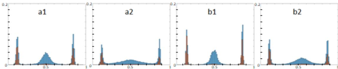
Figure 3.17. Midplane PDFs of *PNT57* ( $\kappa = 0.09625$ ,  $\lambda = 1.5$ ) (a1 and b1) and *PNT35* ( $\kappa = 0.06375$ ,  $\lambda = 1.5$ ) (a2 and b2) suspensions flowing at  $Re = 116$ . The tests are done at  $X/H = 500$  (a1 and a2) and 750 (b1 and b2). In addition, the suspensions have the same number of particles ( $\Phi_{eq} = 0.1\%$ ). The y-axis varies between 0 and 0.2.
