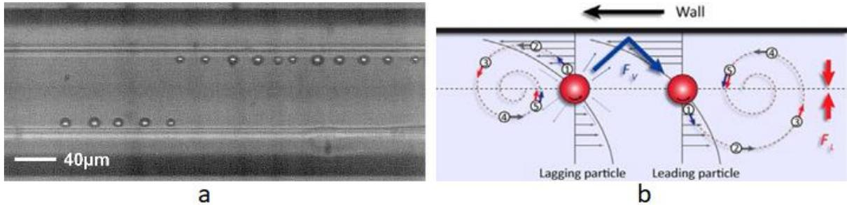
Figure 1.6. (a) A captured image representing the longitudinal ordering of spherical particles in a square channel at  $Re = 210$  (reprinted from [67]); (b) Schematic drawing of the interaction between two aligned particles (reprinted from [68]).
