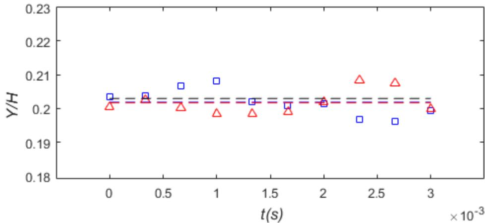
Figure 3.15. Trajectories ( $Y/H$ ) of two SNW particles (red triangles and blue squares) in function of time at  $X/H = 1000$ . The suspension ( $\Phi_{eq} = 0.05\%$ ) is flowing at  $Re = 5.84$ . The normalized equilibrium position is equal to 0.203 (dashed black line). The mean values about which the particles oscillate are represented by the dashed red and blue lines, that are approximately superposed.
