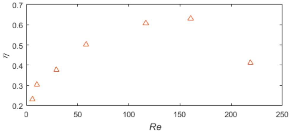
Figure 3.7. Focusing degree in function of the channel Reynolds number for *PNT57* particles ( $\lambda = 1.5$  and  $\kappa = 0.09625$ ). The equivalent particle volume fraction is 0.1% and the tests are done at  $X/H = 1000$  in an  $80\mu\text{m}$  square microchannel.
