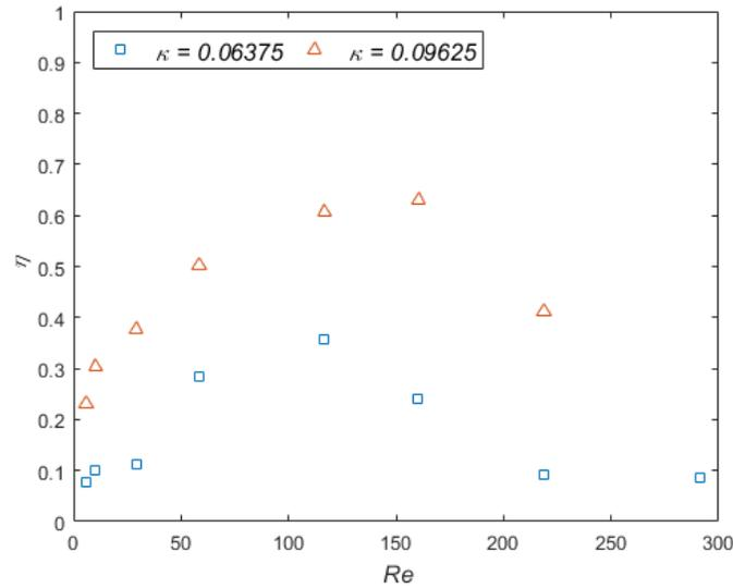
Figure 3.18. Focusing degree in function of Reynolds number for *PNT* particles ( $\lambda = 1.5$ ). The triangles and squares correspond to *PNT57* and *PNT35* particles respectively. Both suspensions have the same number of particles ( $\Phi_{eq} = 0.1\%$ ) and the tests are done at  $X/H = 1000$  in an  $80\mu\text{m}$  square microchannel.
