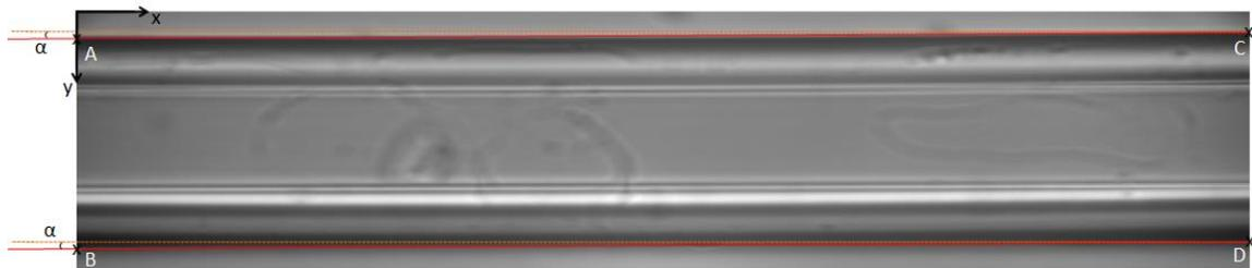
Figure 2.19. The identification of the external walls ( $AC$  and  $BD$ ) as well as the inclination of the channel  $\alpha$ , using the calculated background. The orange line is horizontal, while the red line is inclined by  $\alpha$ .
