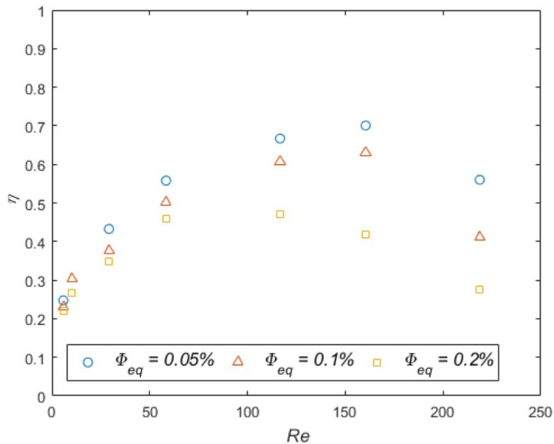
Figure 3.10. Focusing degree in function of the channel Reynolds number for three different equivalent particle volume fractions. The tests are done on PNT57 particles ( $\lambda = 1.5$  and  $\kappa = 0.09625$ ) at  $X/H = 1000$ .
