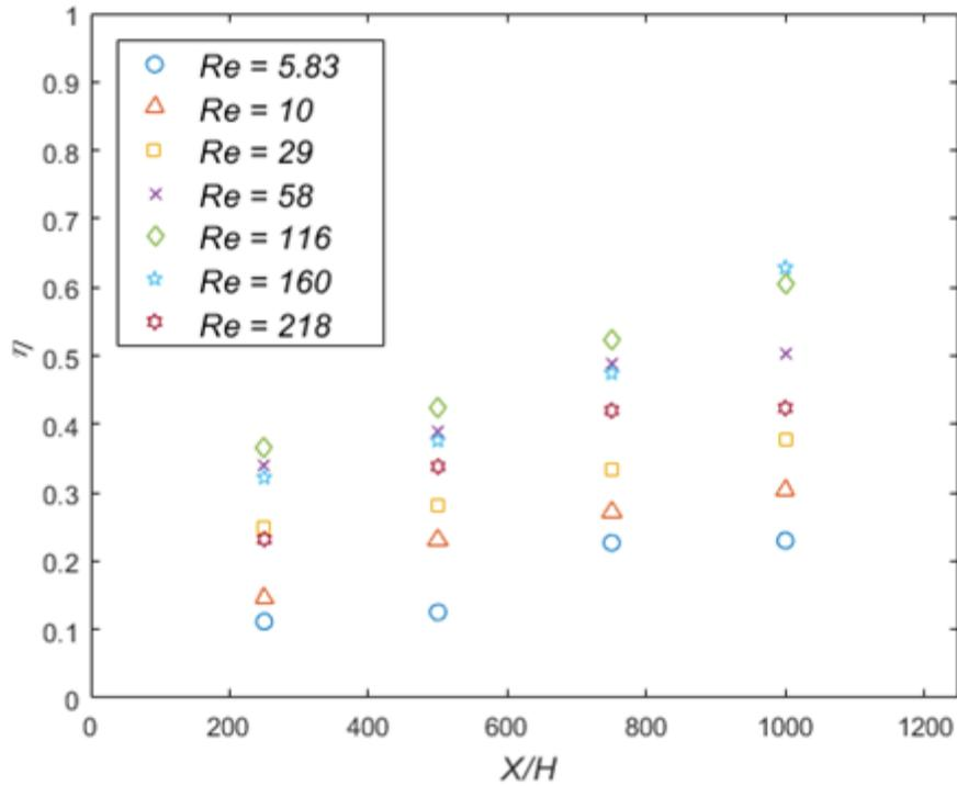
Figure 3.3. Focusing degree in function of the distance from the channel inlet for different values of Reynolds number. The tests are done on a suspension of PNT57 particles ( $\lambda = 1.5$  and  $\kappa = 0.09625$ ), having an equivalent particle volume fraction of 0.1%.
