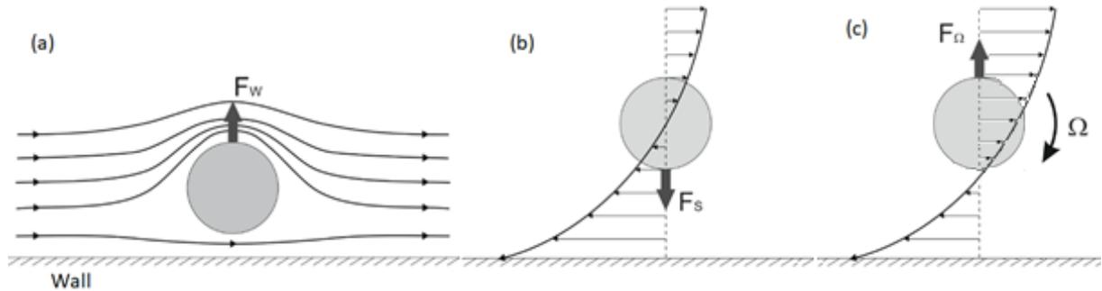
Figure 1.5. Illustration of (a) the wall-induced lift force  $F_W$ , (b) the shear-induced lift force  $F_S$ , and (c) the rotation-induced lift force  $F_\Omega$ . Figures (a) and (b) are reprinted from [67].
