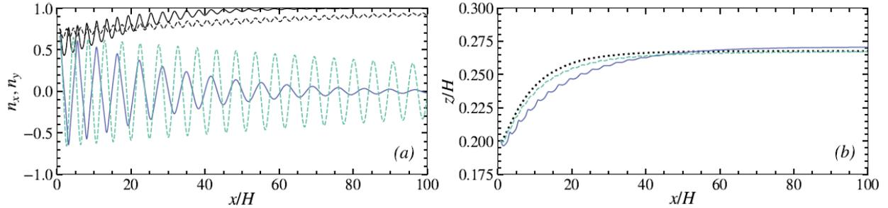
Figure 1.15. (a)  $x$ -components (colored curves) and  $y$ -components (black curves) of the orientation vector of an oblate and (b) trajectories for spheroids with  $\kappa = 0.15$  and  $\lambda = 0.5$  (solid), 0.8 (dashed), and 1 (dotted). Reprinted from [109].
