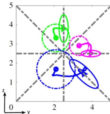
Figure 1.20. Lateral trajectories of oblate rigid particles of different sizes in a square duct at  $Re = 100$ . The particles have the same aspect ratio (ratio between the particle axes,  $\lambda = 1/3$ ) and different volumes. The confinement ratios  $\kappa$
