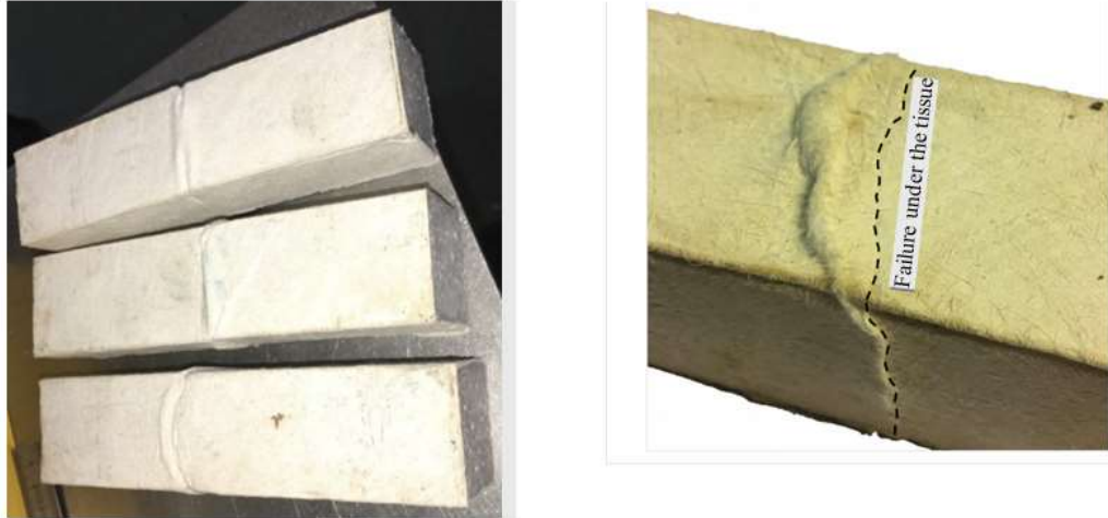
Figure 4- 10: Cracking patterns of mortar prisms (3-Sides)
