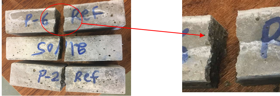
Figure 4- 5: Cracking patterns of mortar prisms (Ref)
