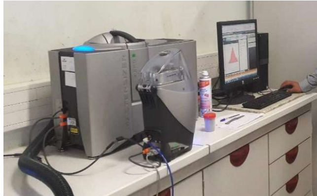
Figure 2- 7: Equipment of the laser diffraction test
