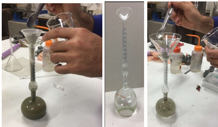
Figure 1: Test procedure for specific gravity of cement
