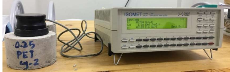
Figure 2-17: ISOMET 2104 equipment for thermal conductivity
