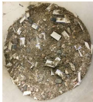
Figure 2- 10: Mix of non-woven cut pieces within the sand
