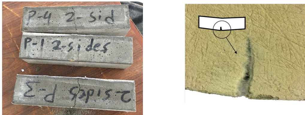
Figure 4- 9: Cracking patterns of mortar prisms (2-Sides)
