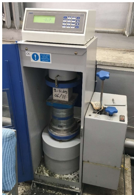
Figure 2- 15: Compressive strength machine used in KPU
