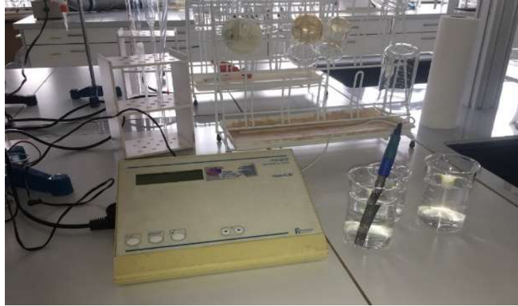
Figure 3: Apparatus for pH value of water
