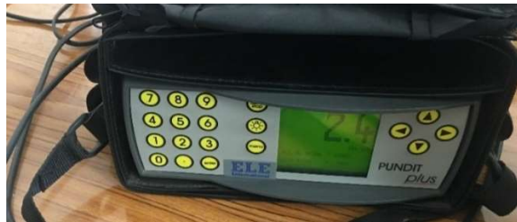
Figure 2- 16: Ultrasonic pulse velocity test equipment
