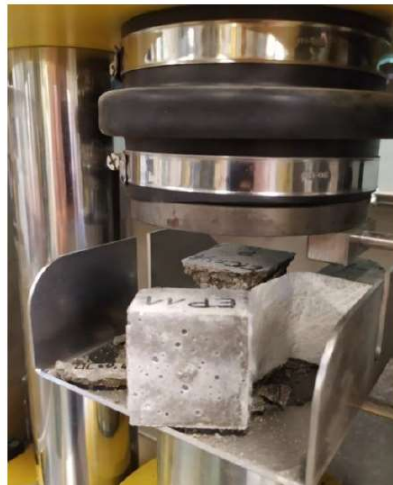
Figure 4- 58: Compressive strength test of samples after bond test
