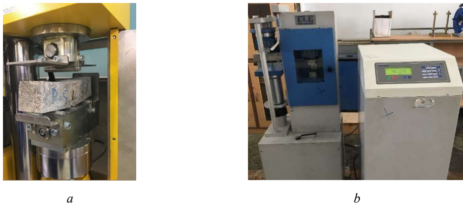
Figure 2- 13: Flexural testing machine: a) INSA and b) KPU
