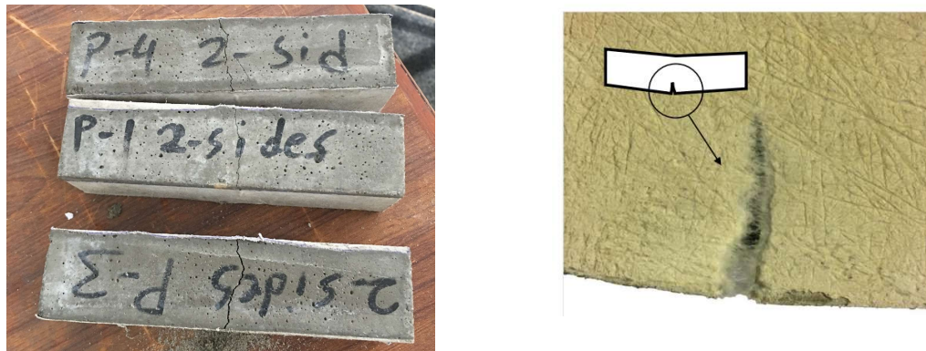
Figure 4- 9: Cracking patterns of mortar prisms (2-Sides)
