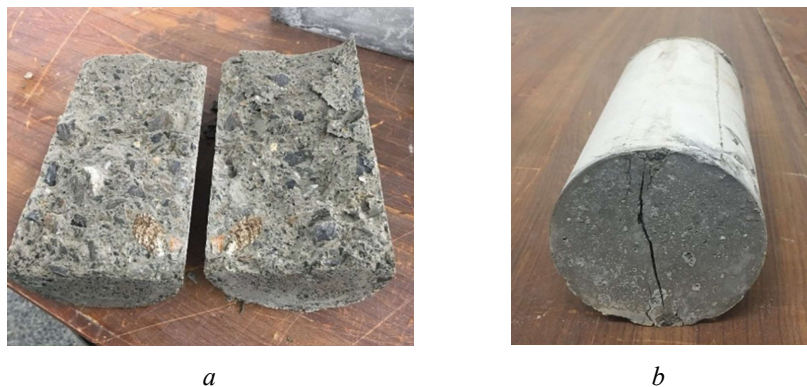
Figure 5- 13: Cracking pattern after tensile splitting testing a) Ref and b) covered samples
