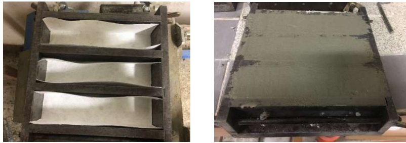
Figure 2- 11: Casting of samples
