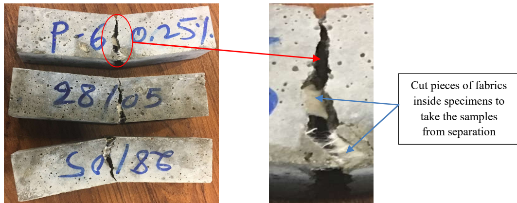
Figure 4- 28: Cut pieces inside the prism
