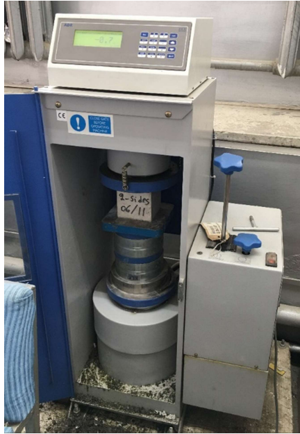
Figure 5: Compressive strength machine in KPU
