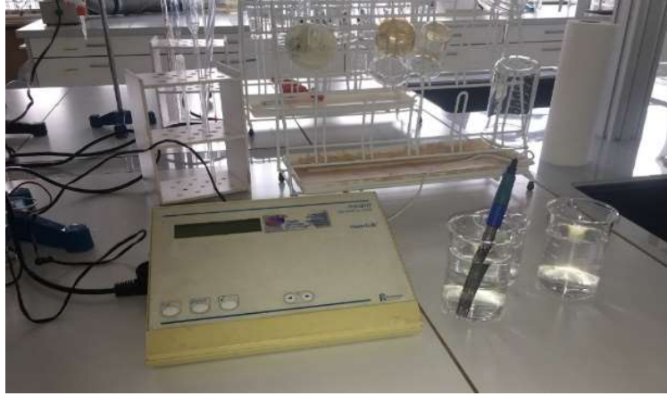
Figure 3: Apparatus for pH value of water
