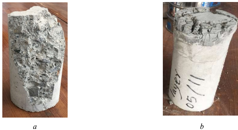
Figure 5- 5: Cracking patterns after compressive strength a) Ref and b) full wrapped samples
