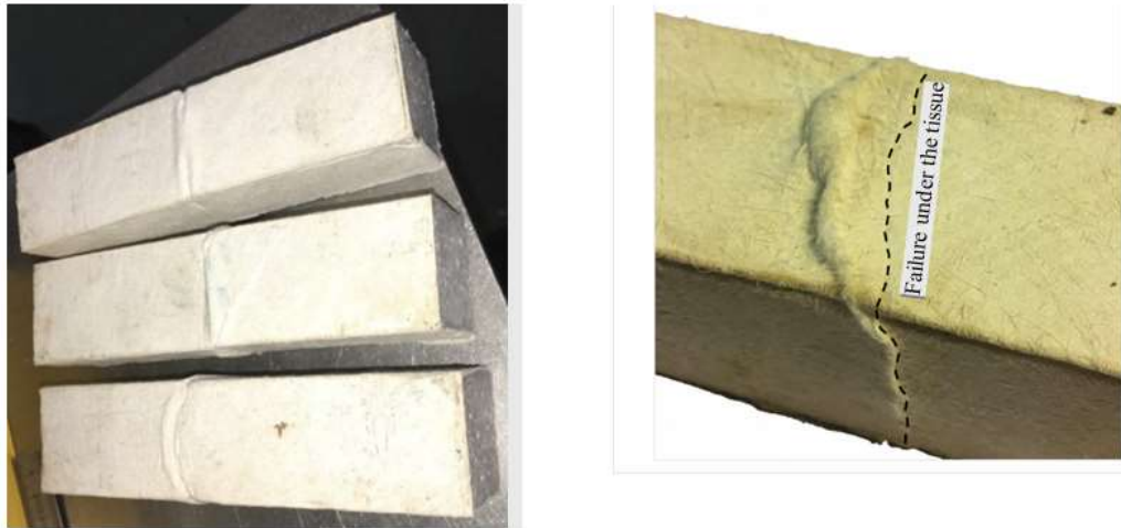
Figure 4- 10: Cracking patterns of mortar prisms (3-Sides)
