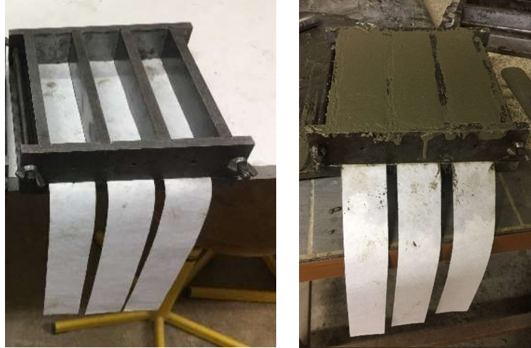
Figure 2- 19: Placement of non-woven sheets in prisms
