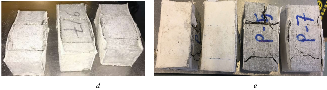
Figure 4- 14: Cracking pattern of mortar samples a) Ref, b) 1-Layer, c) 2-Layers, d) 2-Sides, and e) 3-Sides
