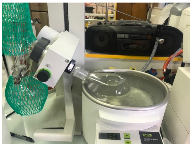
Figure 88. Acetic acid is being removed with a rotary evaporator.
