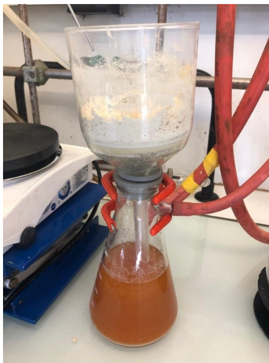
Figure 89. Washing and filtration process with Büchner.
