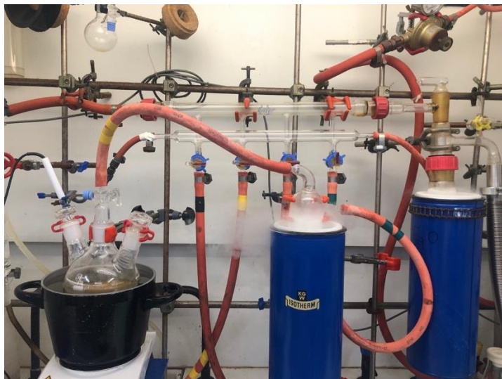
Figure 85. Evaporation step trap by trap.
