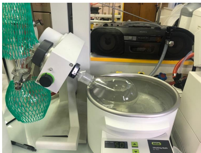
Figure 88. Acetic acid is being removed with a rotary evaporator.
