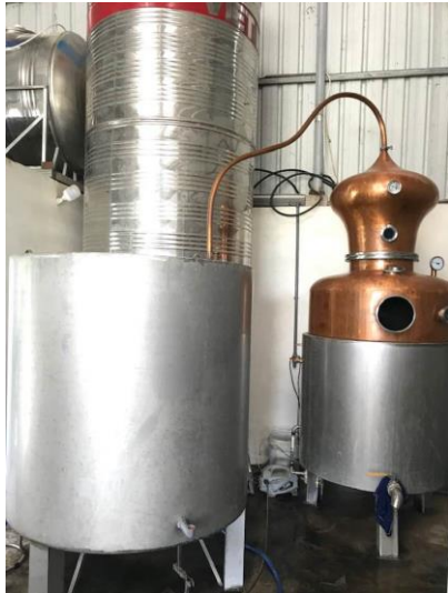
Container - alcohol condensation using water
