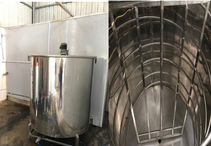
Unique tank for Liquefaction, Saccharification and Fermentation-with an agitator
