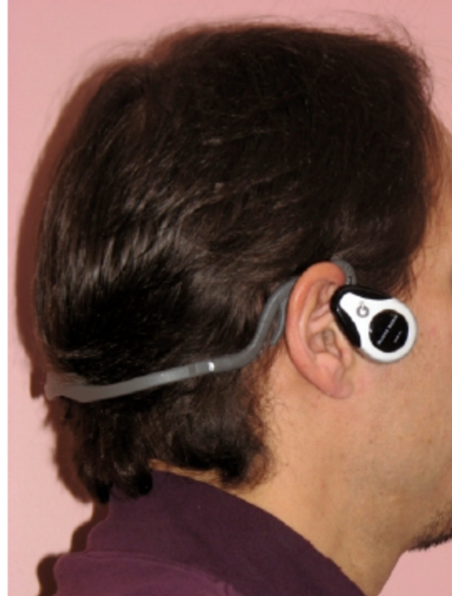
Figure 2.4: Bone-conducting headphones used by Macdonald et al. [105]
