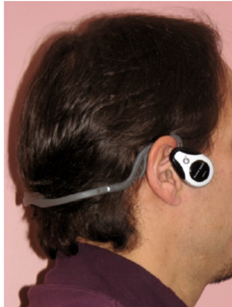
Figure 2.4: Bone-conducting headphones used by Macdonald et al. [105]
