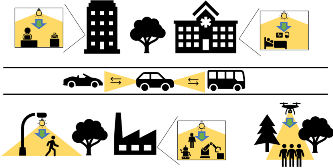
Figure 1.2 — Illustration for different indoor use cases of VLC in rooms/offices and factories (industrial scenarios) to provide high data rate communications, and in hospitals for communications in EMI-sensitive scenarios. Shown also are outdoor use cases of VLC in inter-vehicular communications, communications using streetlights, and communications using UAVs in remote and hard-to-reach areas.
