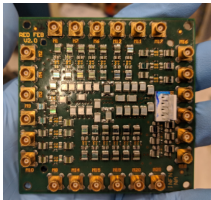
Figure 3.4.4: Top view of the FEB for the top tile, custom developed from INFN Naples together with DarkSide Bologna and LNGS. It is possible to see the 24 read-out channels, four for side, which assured to ReD the best x-y reconstruction available.
