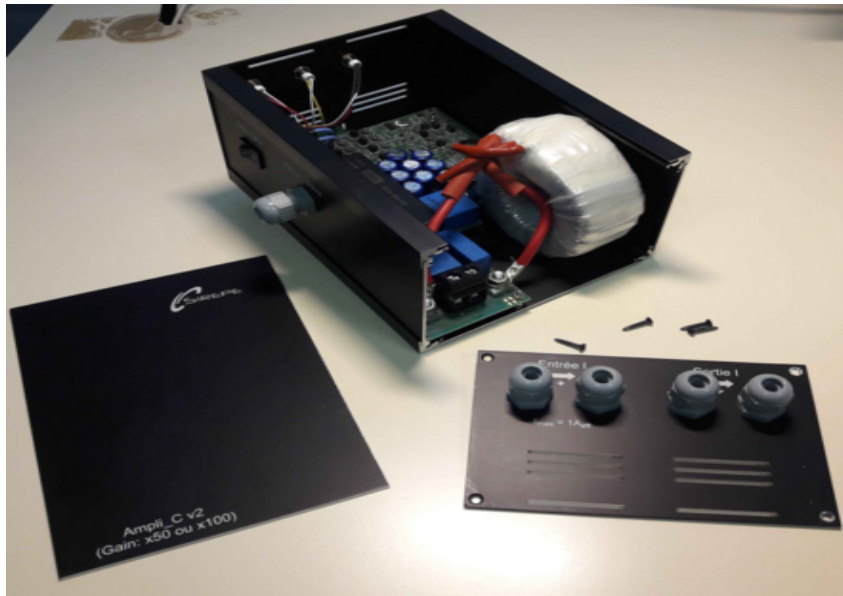
(b) Custom-made “current loop” device used in the setup.
