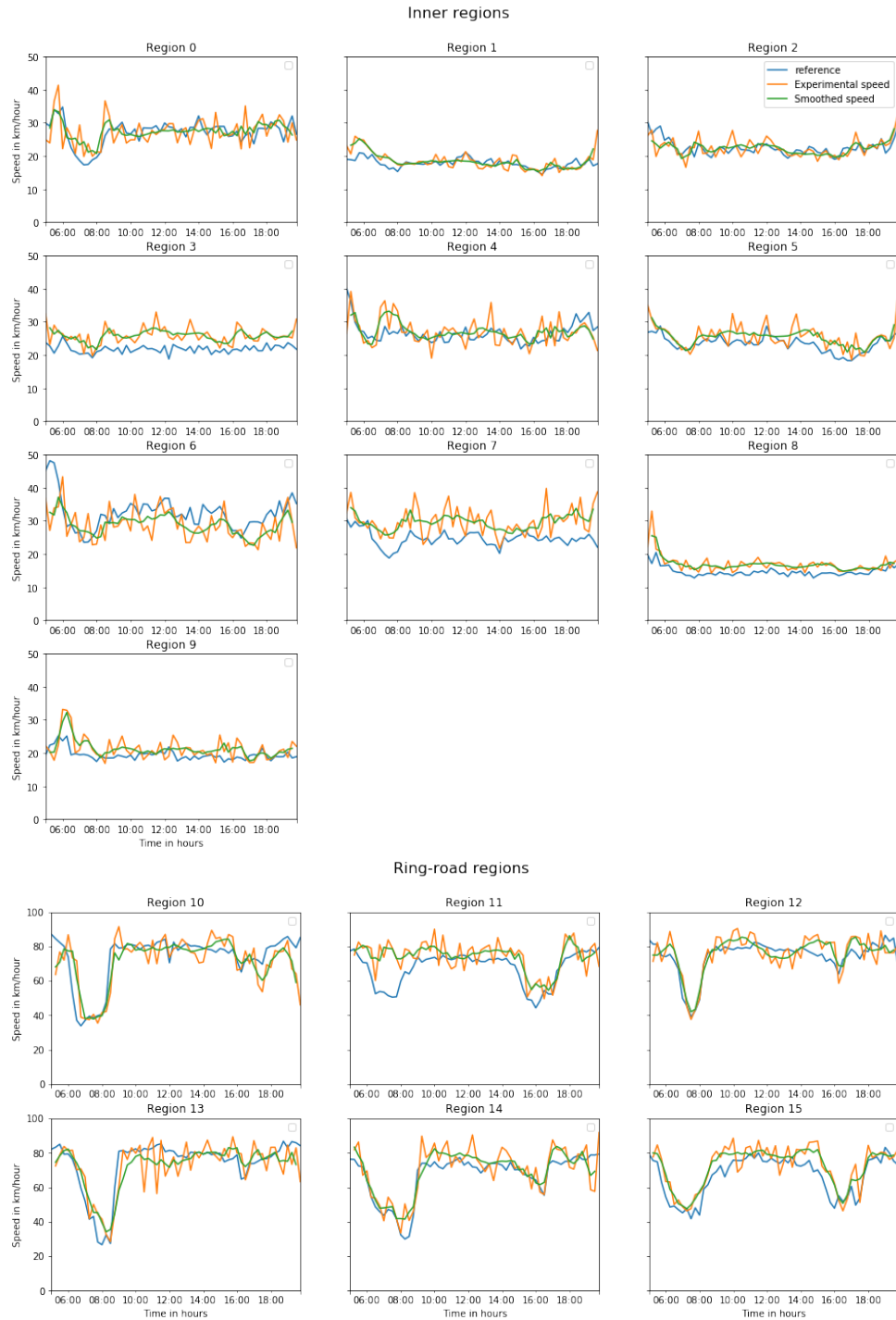
Figure 5.7: Speed estimation method applied to dataset DS_0 (trips with exact travel times), using the dynamic trip lengths
