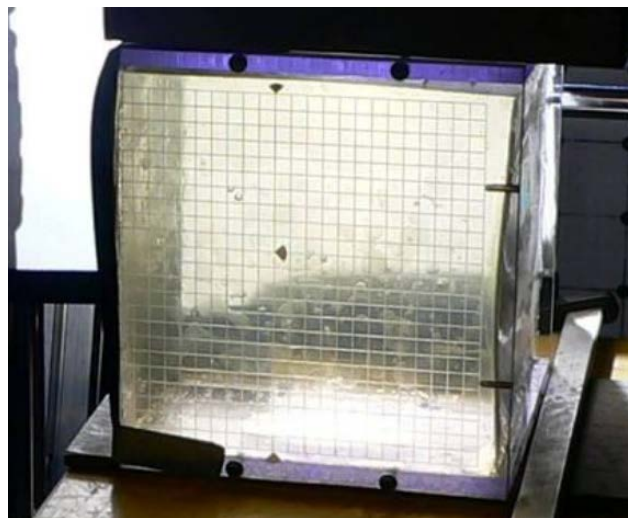
Figure 1.8: Illustration of prototype SEBS gel block [55].
