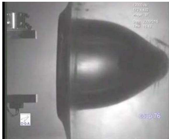
(a) Impact of LLKE projectile on SEBS gel.
