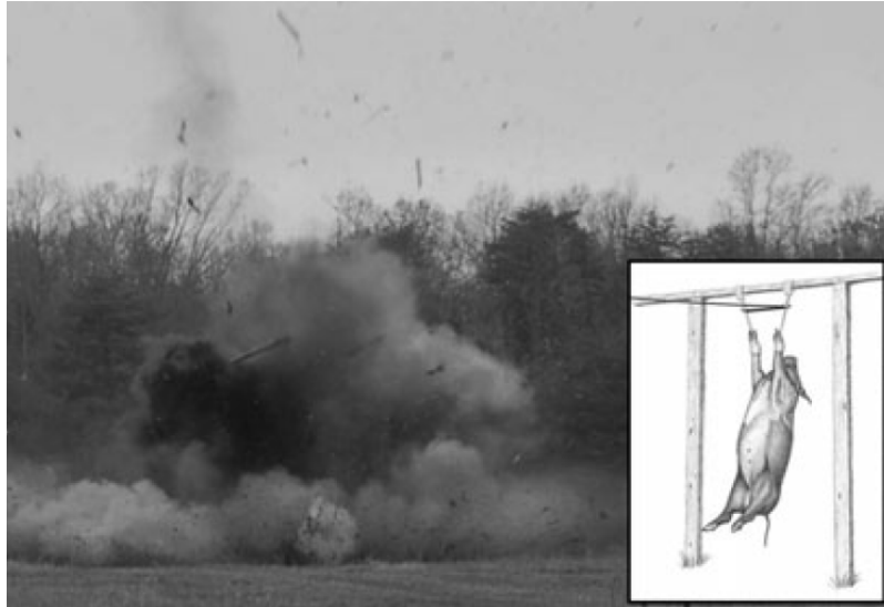
Figure 1.22: Schematic of pig specimen under blast loading, extracted from [82].
