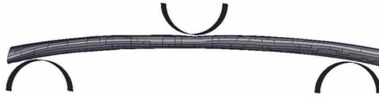
Figure 1.39: Representation of finite element modeling of rib cortical bone under 3PB bending by Charpail [123].
