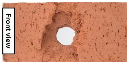
Figure 1.6: Illustration of clay brick impacted by spherical steel spheres [43].
