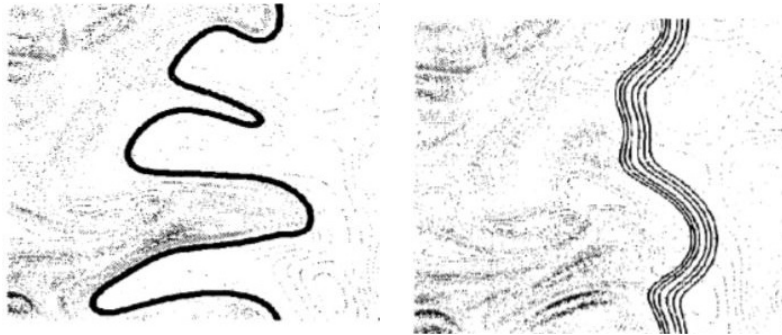
Figure 2.5: DNS of flame turbulence interactions. Reaction rate and vorticity fields are superimposed. (left-side) reference flame; (right-side) flame artificially thickened by a factor \mathcal{F} = 5 . Because of the change in the length scale ratio L_t/\delta_L^0 , combustion/turbulence interaction is changed and the thickened flame is less wrinkled by turbulence motions. This effect can be parametrized using a subgrid scale model (Poinsot and Veynante, 2012).
