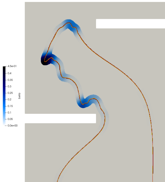
Figure 6.12: Zoom in of a screenshot of LES 3 representing the local wrinkling factor exponent and the flame contour at 35.8 ms. (Blue color map): wrinkling factor exponent and (—): flame contour such as \tilde{c} = 0.5 .
