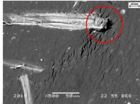
Figure 1-36: Micrographs of a PP/Flax injected sample under loading, the red circle highlighting a high shear stress zone due to the presence of a flax fibres extremity, extracted from [220].
