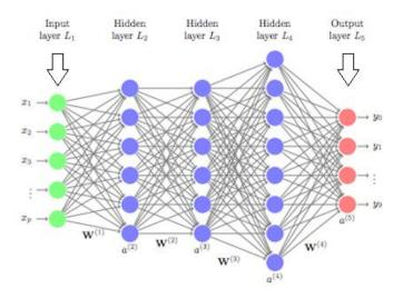
Figure 10: **Illustration of a neural network**: The signal x is put in the first layer and transformed through the successive layers. By adjusting the weights W iteratively, the model is trained to detect automatically the features of the signal that allow a correct classification into one of the classes y in the output layer.
