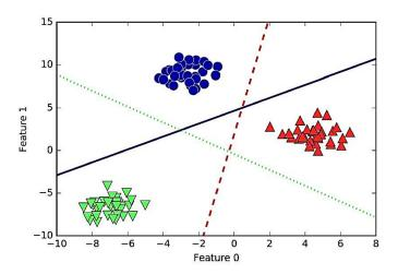
Figure 9: A classification model based on handcrafted feature extraction. Each observation belongs to one of three classes (here physical behaviors), marked with different shapes and colors. Based on two features defined and computed by the researcher (feature o and feature 1 - e.g. the mean and the median of the signal over the window), a good classification model draws decision boundaries that separate the plane into decision areas corresponding to each class (Adapted from [79])
