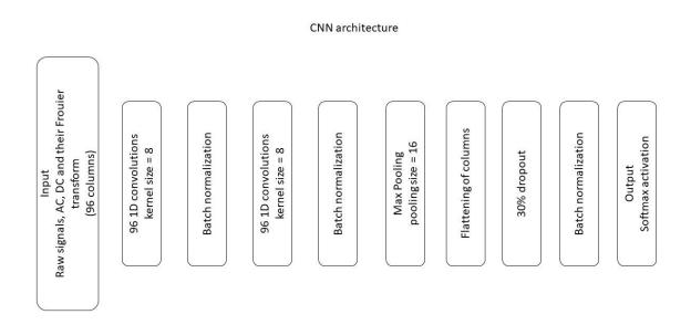
Figure 2: The **Convolution Neural Network** tested here. Except for the output, all layers were activation with the RELU function.
