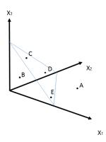
Figure 4: **Representation of a 2-D simplex in the real 3-D space**. All three-part compositions (x1, x2, x3) lie on the triangle (simplex), because of the constraint of adding up to 1. Points C, D, and E are therefore possible compositions, but not A and B. Compositional analysis acknowledges the constrained sample space of the compositions (and thus their interdependency). In contrast, in classical regression models view each part belongs to the unconstrained real space.
