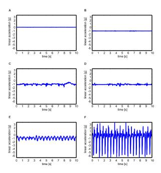
Figure 8: **Example of raw accelerometer signal** (hip, sagittal axis) for different behaviors. (A) Lying, (B) Standing, (C) Vacuuming, (D) Sweeping, (E) Walking, (F) Rope jumping. Models aim to classify behaviors based on the difference in the patterns of the signals (Image from [73]).
