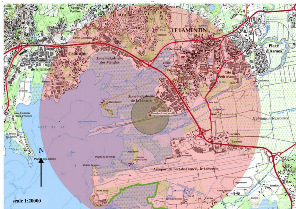
Figure 13: Localisation of a potential reinjection well according to the level of considered exigencies (criterion -20m, but with a more important flow Q = 0.02 \text{ m}^3/\text{s} ).
