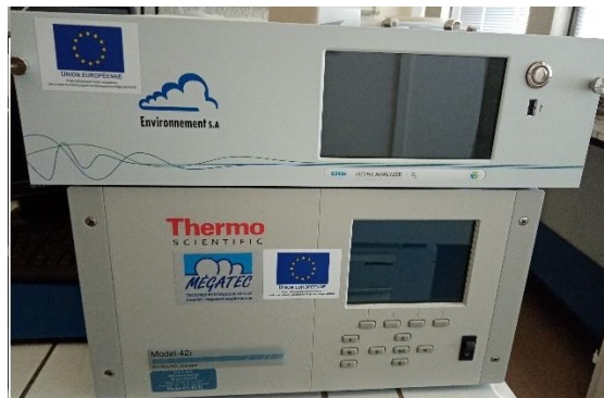
Figure 32 The NO x (bottom) and the O 3 (top) analyzers used in our experiments.
