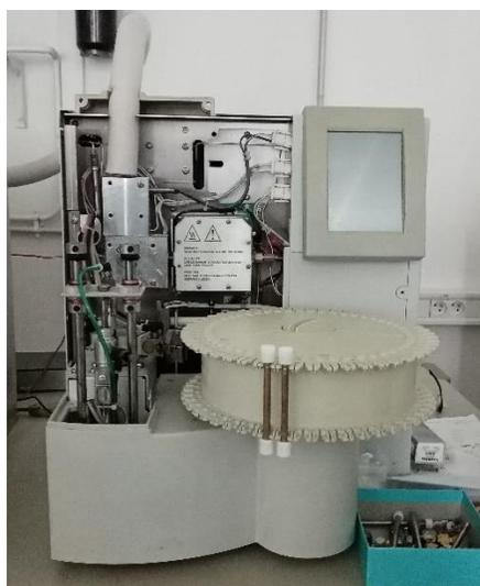
**Figure 30 ATD (automated thermal desorption) system.**
