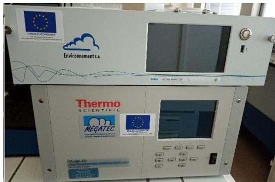
**Figure 32** The NO<sub>x</sub> (bottom) and the O<sub>3</sub> (top) analyzers used in our experiments.
