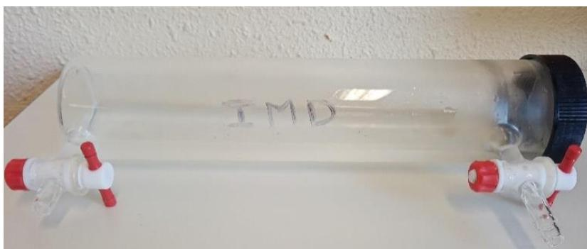
**Figure 33** IMD solution in the glass reactor.
