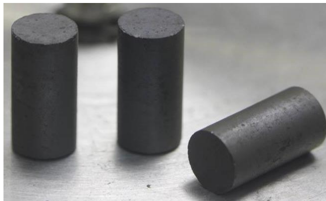
Figure 1-3: Fuel pellets of U_{0.71}Pu_{0.28}Am_{0.01}O_{1.98} for SFR (height: 11 mm – diameter: 5.4 mm).
