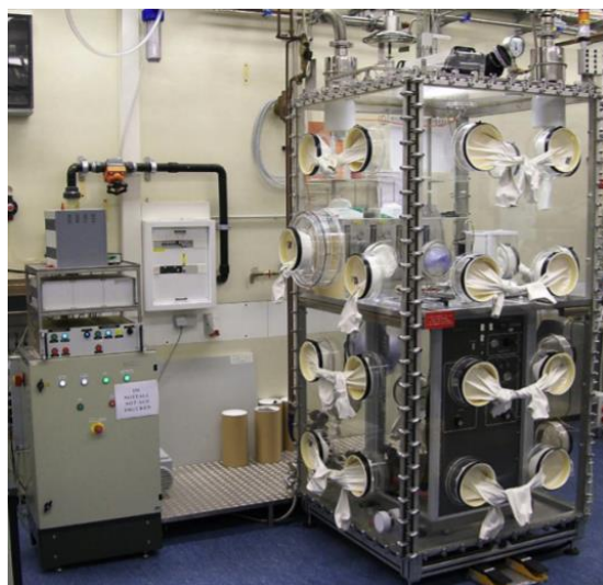
Figure 3-8: Drop calorimeter installed in a glovebox at JRC-Karlsruhe (left box: electronics parts) [224].
