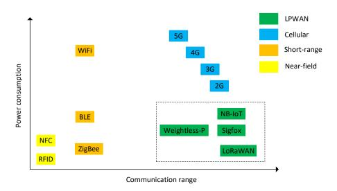
Figure 1.1 – Power consumption versus communication range for various radio protocols, as depicted in [5].
