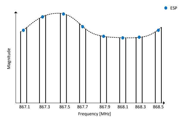
Figure 4.14 – Estimating the wide-band CSI shape by either integrating the narrow-band CSI shapes or the ESP values of the frequency bands.
