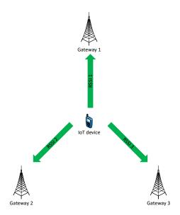
Figure 2.4 – Example of localization based on RSSI.
