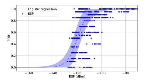
(a) Measured PDR versus different ESP values.
