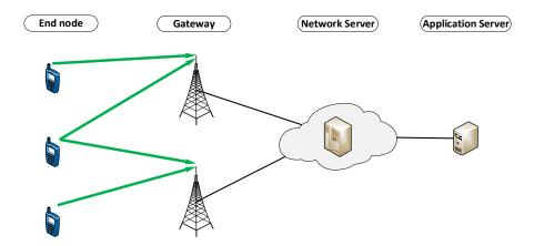
Figure 2.3 – General LoRaWAN architecture.
