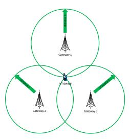
Figure 2.5 – Example of localization based on trilateration.
