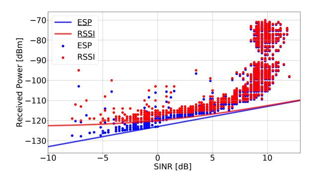
Figure 4.10 – Comparison of the measured RSSI and ESP against SINR.
