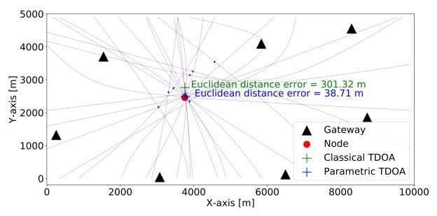
Figure 3.1 – A sample pattern from the algorithm ( $\rho = 2.5 \,\mathrm{km}$ ,  $wid = 10 \,\mathrm{km}$ ,  $len = 5 \,\mathrm{km}$ ).
