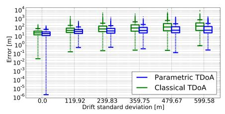
(a) Errors at each value of the drift standard deviation.
