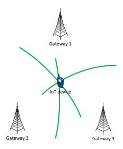
Figure 2.6 – Example of localization based on TDoA.
