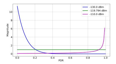
Figure 5.6 – Beta distribution function  $f(PDR; \alpha, \beta)$  at different ESP values.
