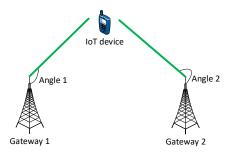
Figure 2.7 – Example of localization based on AoA.
