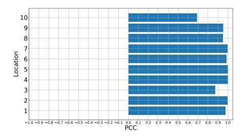
Figure 4.12 – The PCC magnitude between the uplink and downlink CSI at each location.
