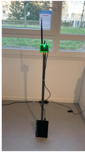
Figure 6.2 – The packaged Pycom device is fixed on a rod and connected to a battery inside a building.
