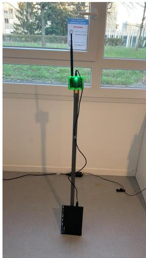
Figure 6.2 – The packaged Pycom device is fixed on a rod and connected to a battery inside a building.
