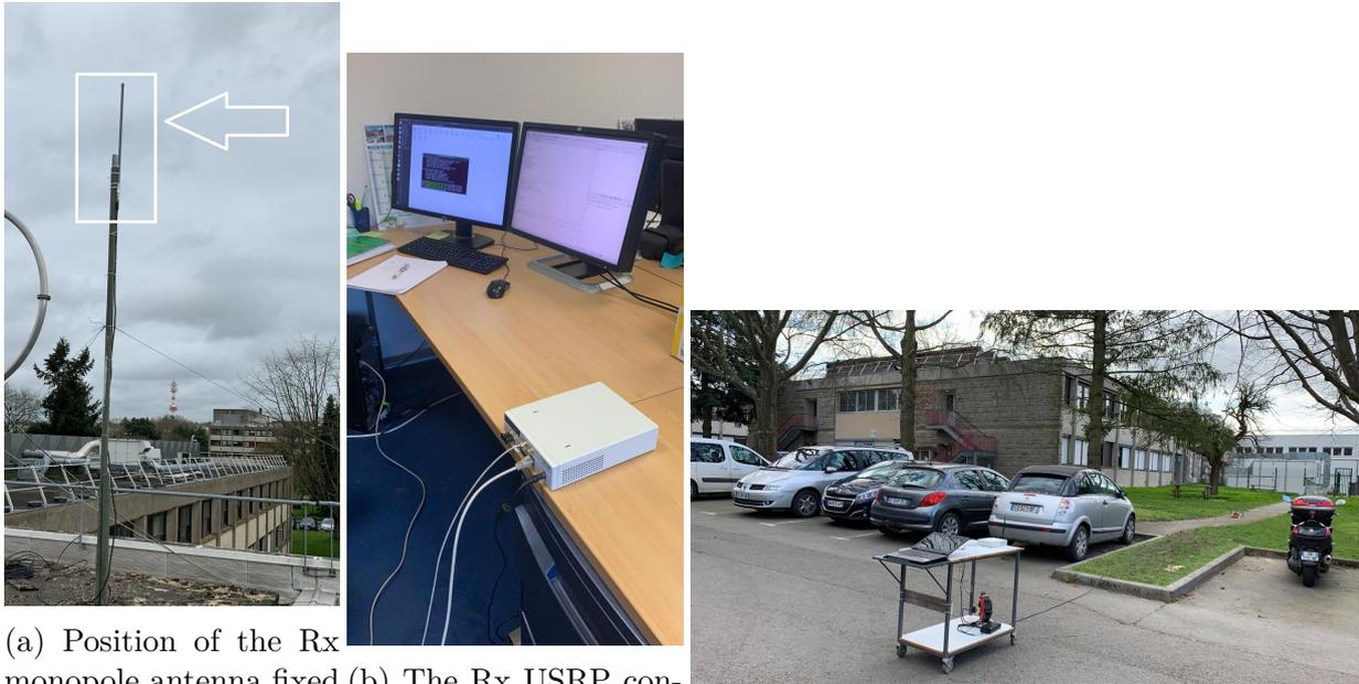
(a) Position of the Rx monopole antenna fixed on the roof of the IETR (b) The Rx USRP connected to the computer and the antenna cable. (c) A trolley shelf with the different parts of the lab transmission equipment at Tx location 2.
