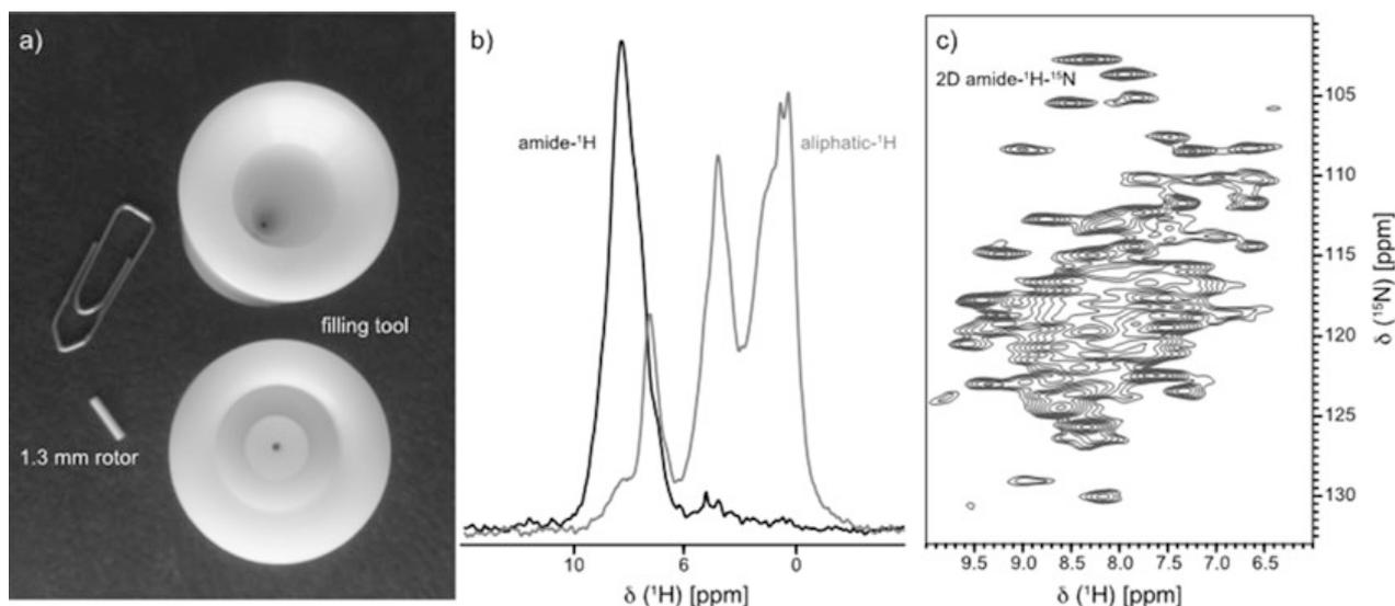
**Fig. 3** Fast-MAS-NMR analysis of hCTR1 in MLVs. (a) 1.3 mm solid-state NMR rotor and filling tool. (b) One-dimensional amide-<sup>1</sup>H (1D 1H-<sup>15</sup>N CP-HSQC) and aliphatic-<sup>1</sup>H (1D 1H-<sup>13</sup>C CP-HSQC) spectra. (c) Two-dimensional <sup>1</sup>H-<sup>15</sup>N CP-HSQC spectrum of <sup>13</sup>C,<sup>15</sup>N labeled hCTR1 in POPC-Cholesterol MLVs recorded on an 800 MHz spectrometer with 60 kHz MAS
