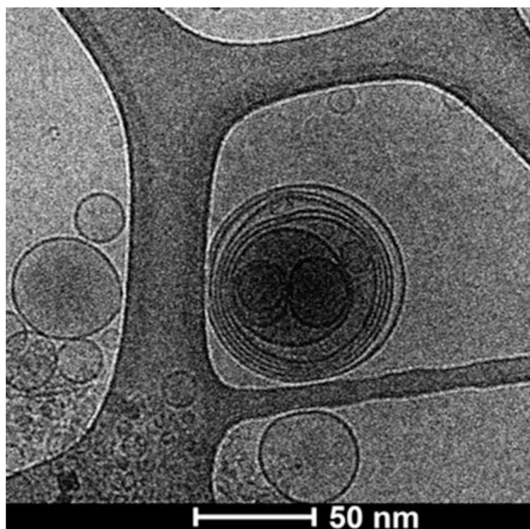
**Fig. 2** Visualization of hCTR1 reconstituted in MLVs by cryo-TEM. MLV sample was blotted on a Lacey carbon film grid with a Vitrobot MARK IV instrument (FEI). Image (28,000 $\times$  magnification) was acquired at 200 kV on a Glacios microscope (ThermoFisher)
