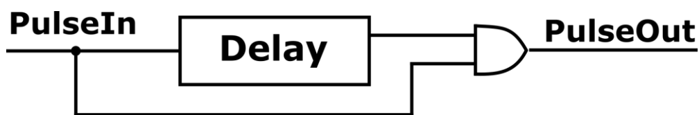
Figure 53: Schematic of the implemented pulse shrinking element.
