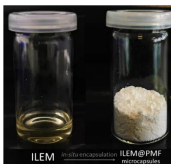
Figure 4-4 ILEM (left) and ILEM@PMF microcapsules (right)
