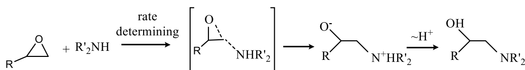
Scheme 3-3 General mechanism for epoxy-amine curing [52]
